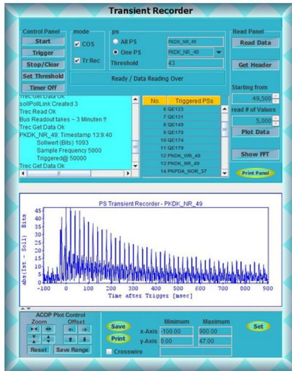
Figure 4: The graphics user interface of PSC Transient Recorder.
