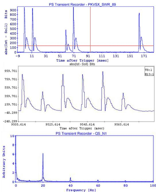
Figure 6: (a) The transients in the PS PKVSX\_SWR\_89, (b) The transients in the PS PKVSU\_SWL\_46 recorded in Transient recorders where the difference in between set & read back current is  $\sim 1000$ bits and (c) shows the frequency spectrum of the transients in PS QS\_N1.
