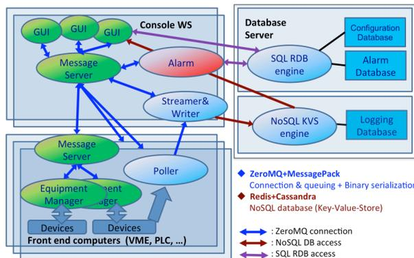
Figure 5: Software structure of MADOCA II that uses ZeroMQ and MessagePack for the message transaction. The NoSQL database engines receive machine status data from the Writer processes.
