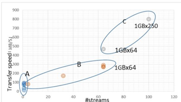
Figure 5: Speed of data transfer from SACLA to HPCI storage [8][9] at RIKEN AICS as a function of the number of parallel streams. A: gsisep protocol (#stream=1), several encryption types; B: gfpcopy protocol with default setting; C: gfpcopy protocol after TCP window size tuning. The highest performance was achieved when 250 1 GB-sized files were transferred using 100 parallel gftp streams.
