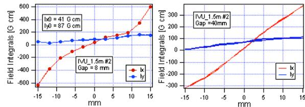
Figure 4: Field integrals of a 1.5m IVU.
