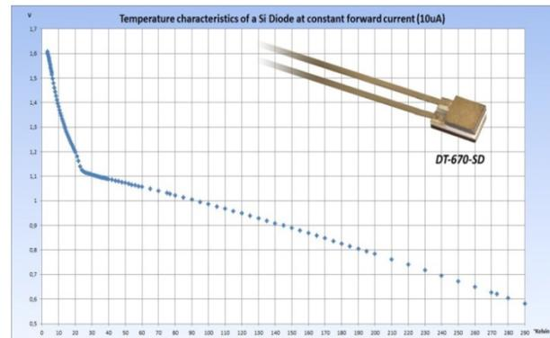
Figure 3: Diode sensor DT 670-SD characteristic curve [5].
