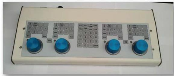
Figure 3: Knob system device realized for managing the magnet system.
