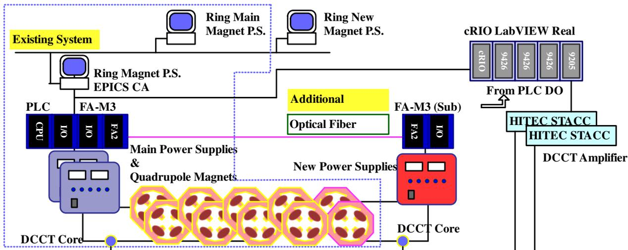
Figure 3: Existing power supplies control system and developing power supplies control system. Sub unit of the PLC is connected by the optical fiber cable to main PLC unit to synchronize to main PLC unit. The external DCCT of the power supplies are also shown. The external DCCT are used for feed-back current control system and accurate monitoring of the power supplies.
