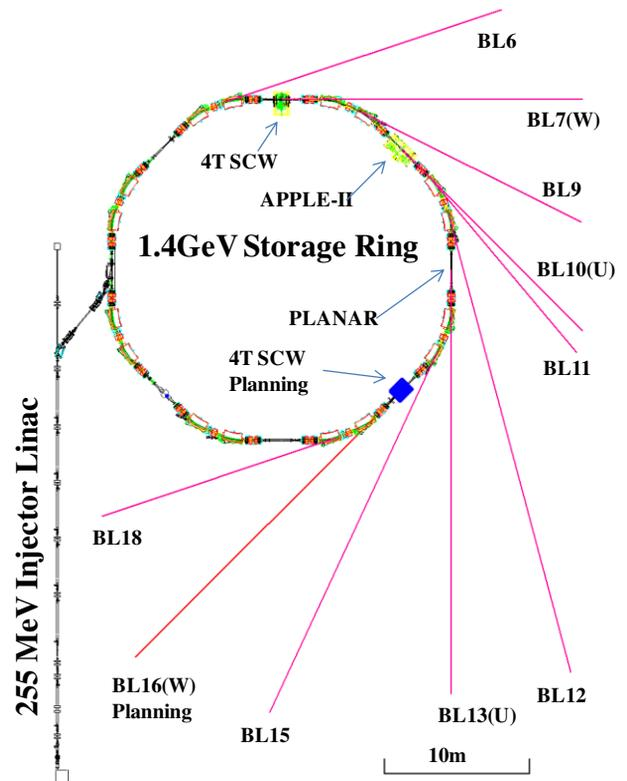
Figure 1: Layout of the SAGA Light Source.
