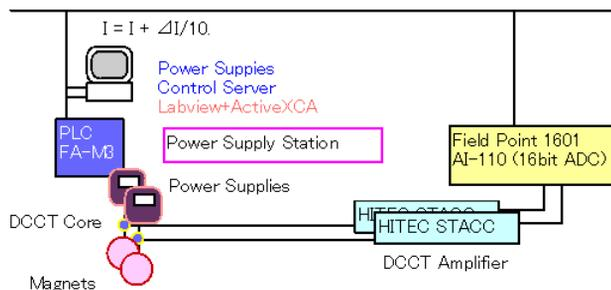
Figure 4: Feed-back Current Control System by External DCCT.
