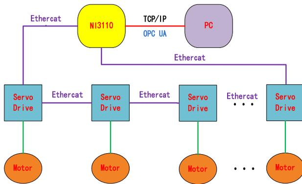
Figure 2: Architecture of motion control system.
