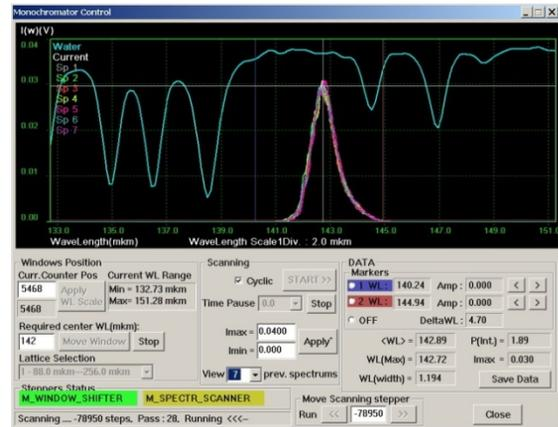
Figure 3: Plot of measured FEL radiation spectrum.
