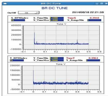
Figure 7: Tune Measurement from BPM TBT data.
