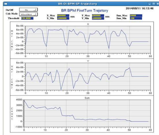
Figure 5: First turn horizontal, vertical trajectory and sum along 60 BPMs of booster.
