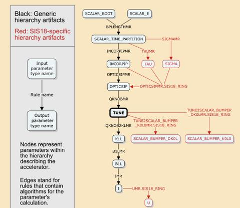
Hierarchy for inputs and outputs of the tune parameter type. Distinctive features of SIS18 added keeping the generic ring accelerator model structure.
