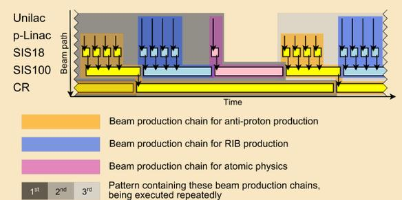
Example for parallel beam operation showing aggregation of beam process chains into patterns. HESR accumulating the anti-protons is omitted.
