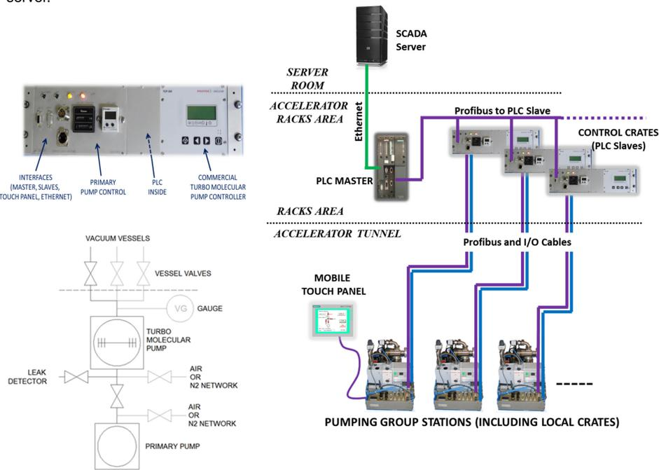
The new control system is compatible with any hardware control crates based on Siemens® PLC S7-300 or S7-400 series with a minimum of 64Kb working memory. The control system is compatible with the recent CERN designed crate shown in Figure 2 but also with the 15 years old crates. Pumping group devices are controlled using direct PLC Input/Output or Profibus® fieldbus.
