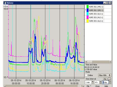
The pumping group pressure gauges history is an additional tool to check pumps efficiency, analyse pumping speed and detect leaks.
