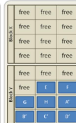
3. In order to write to the pages with stale data (A-D) all good pages (E-H & A'-D') are read and written to a new block (Y) then the old block (X) is erased. This last step is garbage collection.
