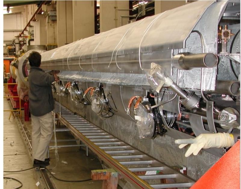
Assembly of thermal radiation shields at DESY
