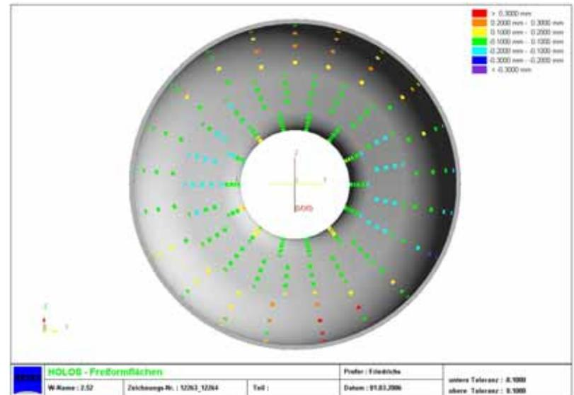
**Shape accuracy:** Optical and mechanical 3D measurement of the half cell shape
