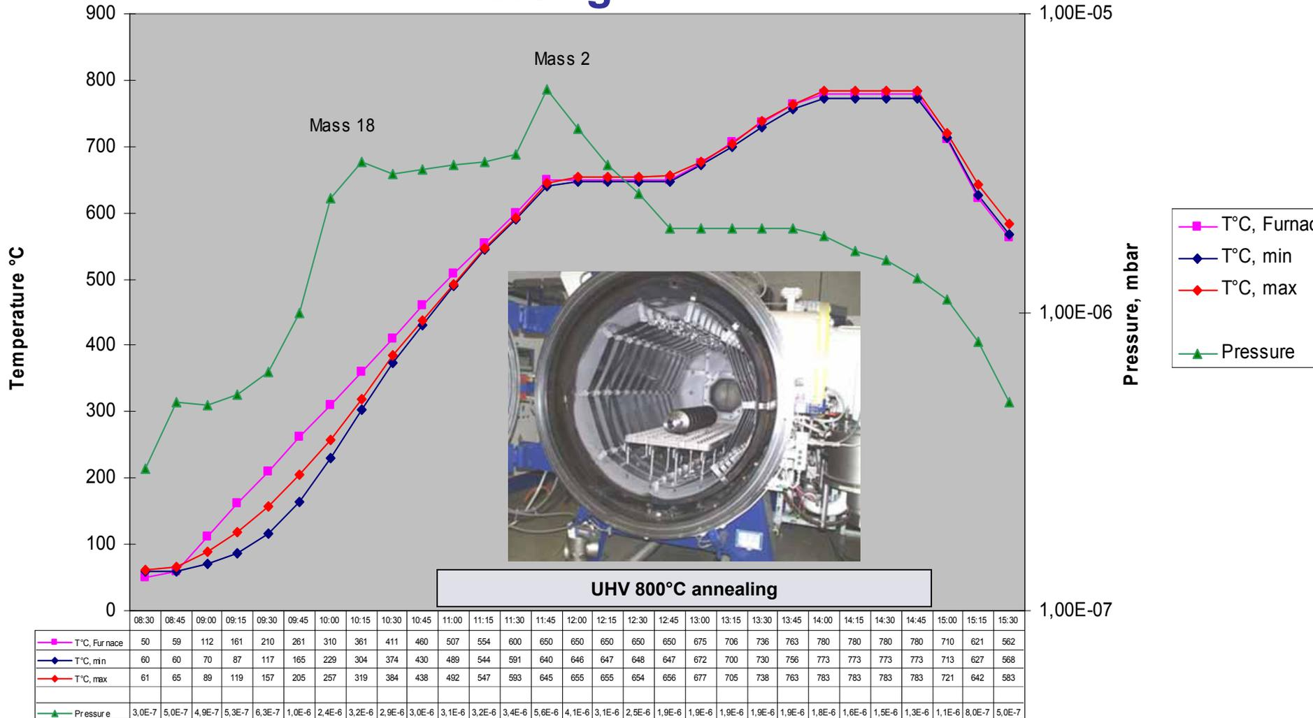
The temperature and the total pressure in the chamber during annealing of Nb300.
