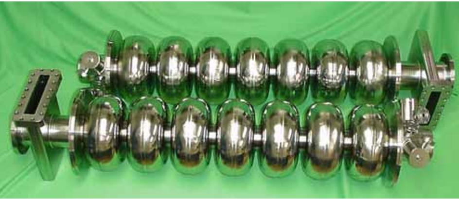
JLab: Two Jlab upgrade **7-cell cavities** are completed from Ningxia/ CBMM large grain Nb
