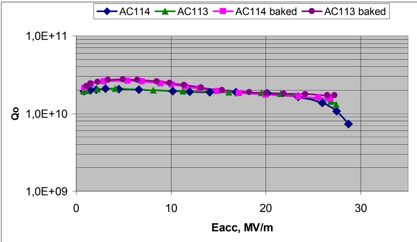
Second test  $Q(E_{acc})$  curve of the LG nine cell cavities AC113-AC114 at 2K after additional 20-30  $\mu\text{m}$  BCP and 125°C, 50 h baking
