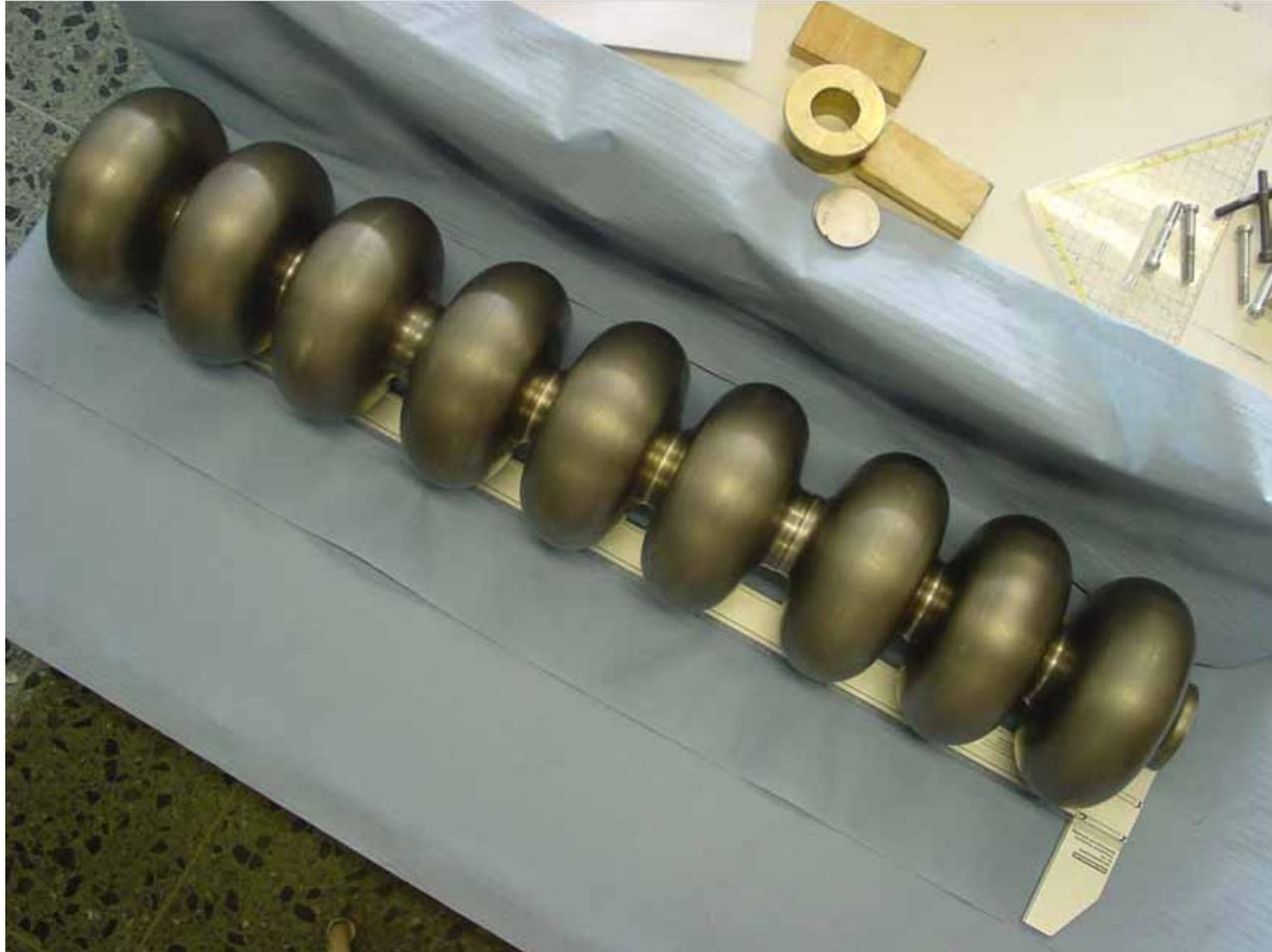
New DESY multi cell units produced by hydroforming
