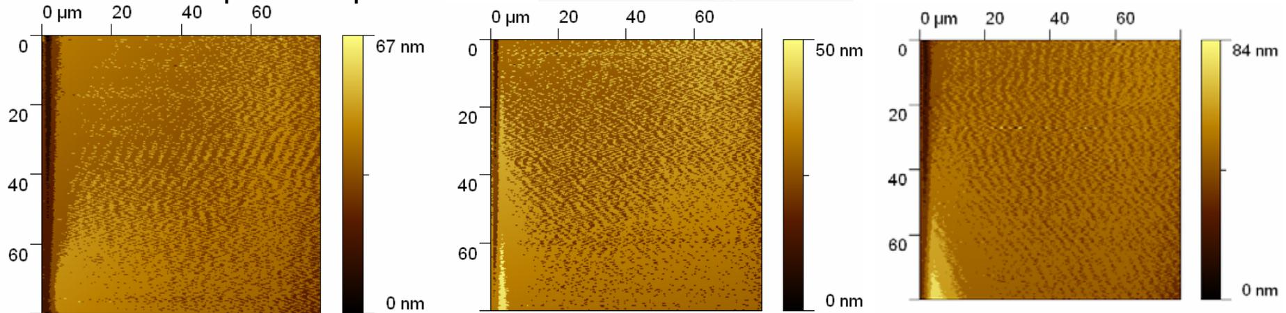
AFM roughness measurement (X. Singer, A. Dangwal-Pandey). Roughness of fine grain Nb after EP is 251 nm (A. Wu) .
