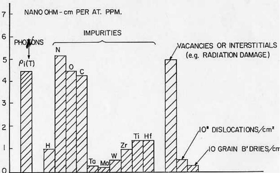
Contribution of different defects in the scattering mechanism (Schulze)
