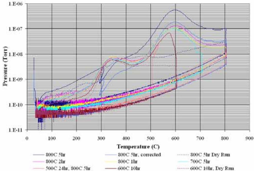
Hydrogen partial pressure versus annealing temperature
