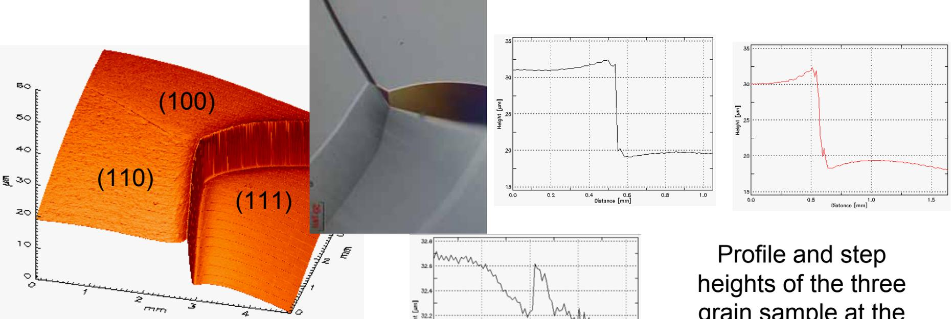
Light microscope and AFM image of LG Nb, BCP etched up to 100 μm
