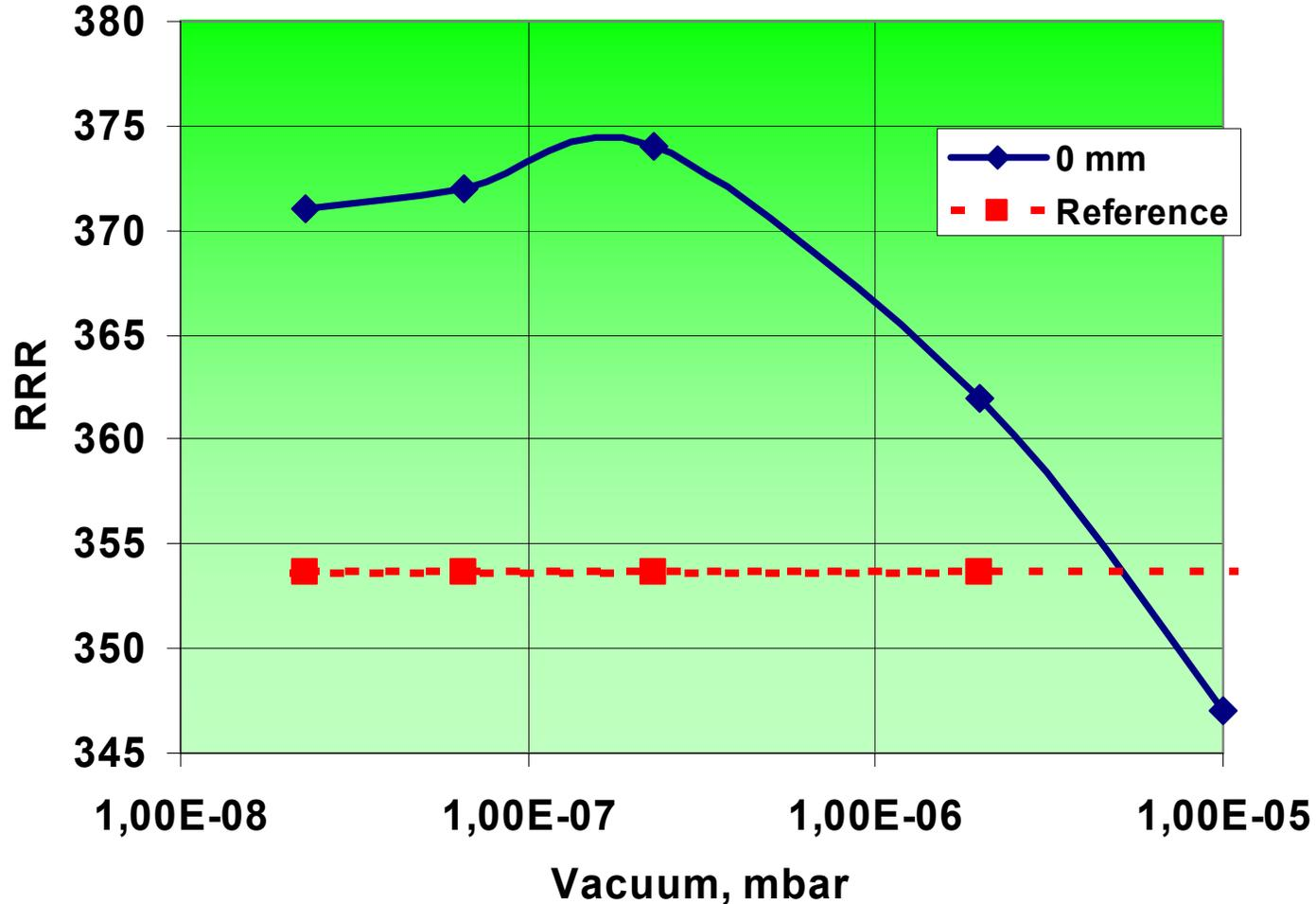
RRR in the welding seam versus pressure in the welding chamber
