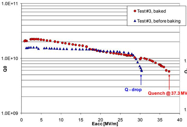
Large Grain TESLA Cavity Shape TD3
