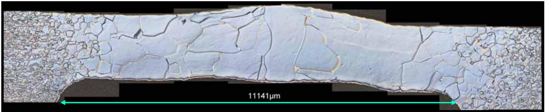
Microstructure of the EB welding area. The grain size
