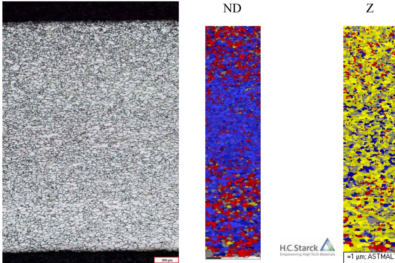
Electron back scattering diffraction EBSD
