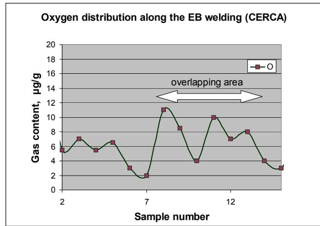
Oxygen distribution along the welding seam. RRR= 280 in the welding seam and RRR= 207 in the overlapping.
