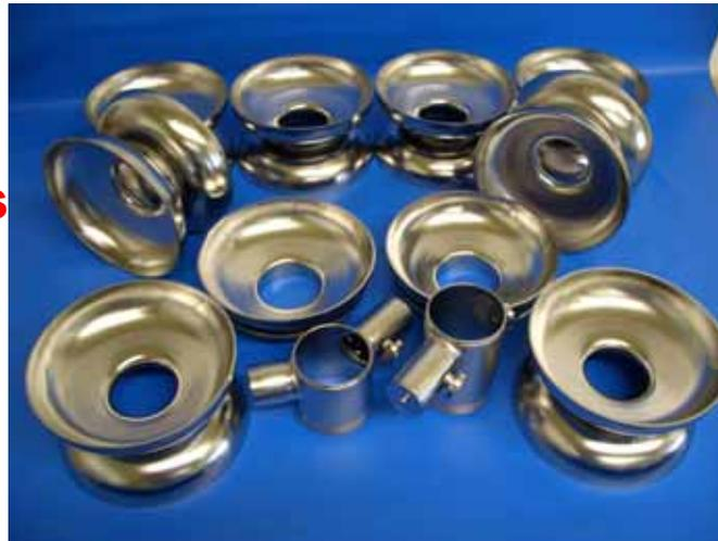
In discs for AC151-AC154, the main orientation of the central crystal is (100), for discs of AC155-AC158 mainly (211) or (221). For the disc with (100) orientation, a more pronounced anisotropy and quadrangular shape after deep drawing was observed. The difficulties for assembling of half cells and dumb-bells for welding have been overcome by using a special tool
