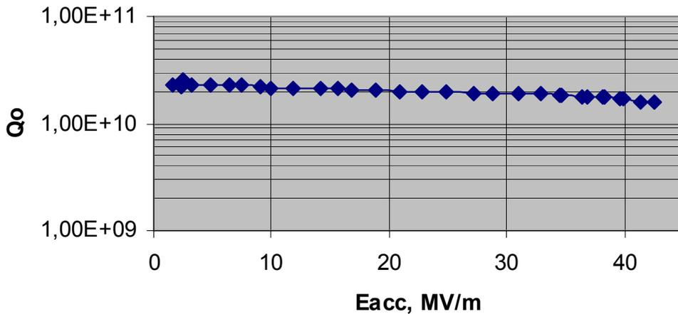
◆ 1K2, Nb100 Heraeus, HT1400°C, BCP 250  $\mu$ m, EP 100 $\mu$ m
