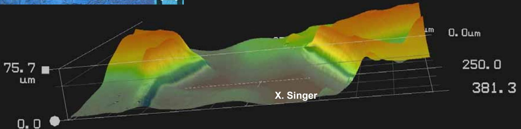
Example of welding connection of EP treated cavity. Up to 75  $\mu\text{m}$  steps
