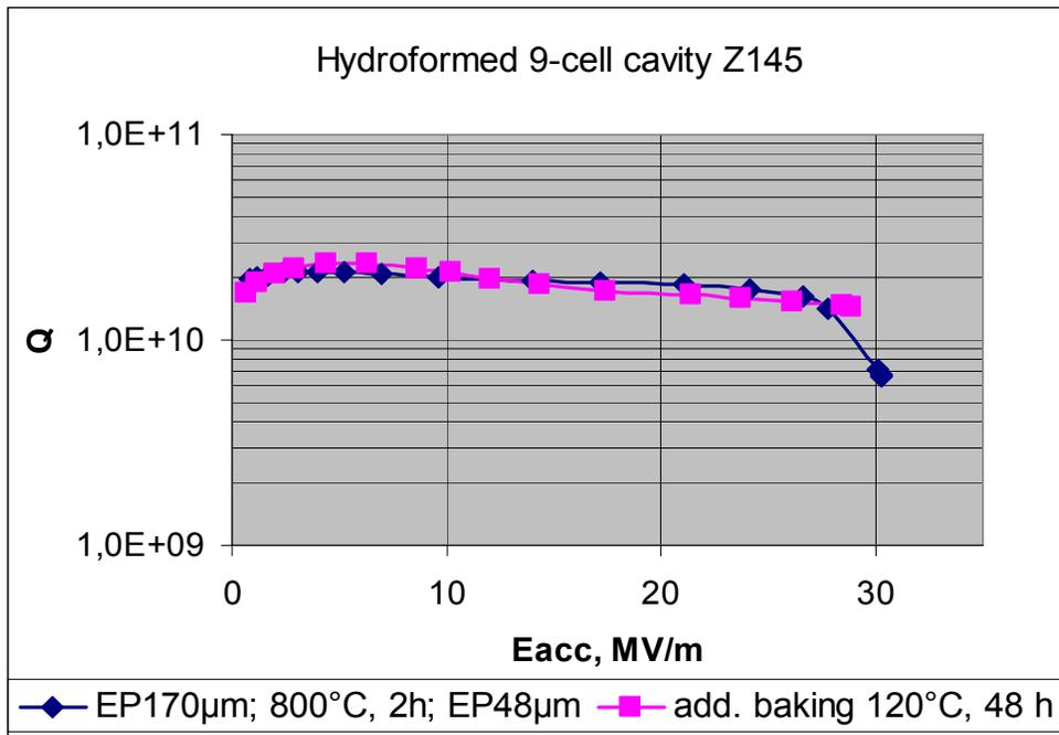
Surface treatment at DESY: 40 mm BCP, 800 °C heat treatment, tuning; 170 mm electropolishing (EP), ethanol rinsing, 800 °C heat treatment; 48 mm EP, HPR, assembly and evacuation. After “in-situ” baking at 120 °C for 48 h. the Q-drop almost disappeared, but the Eacc was not increased. The cavity is welded into the He vessel, will be installed in one of next acc. cryomodules at DESY.
