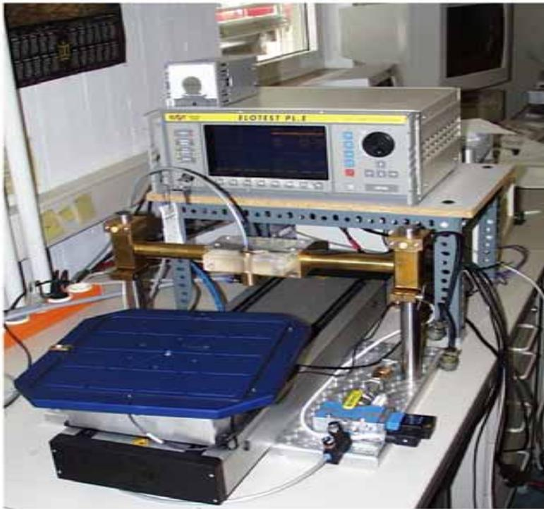
DESY eddy current scanning apparatus for niobium discs. 100% Nb sheets for TTF scanned and sorted out. **Feed back to Nb producer was very important**
