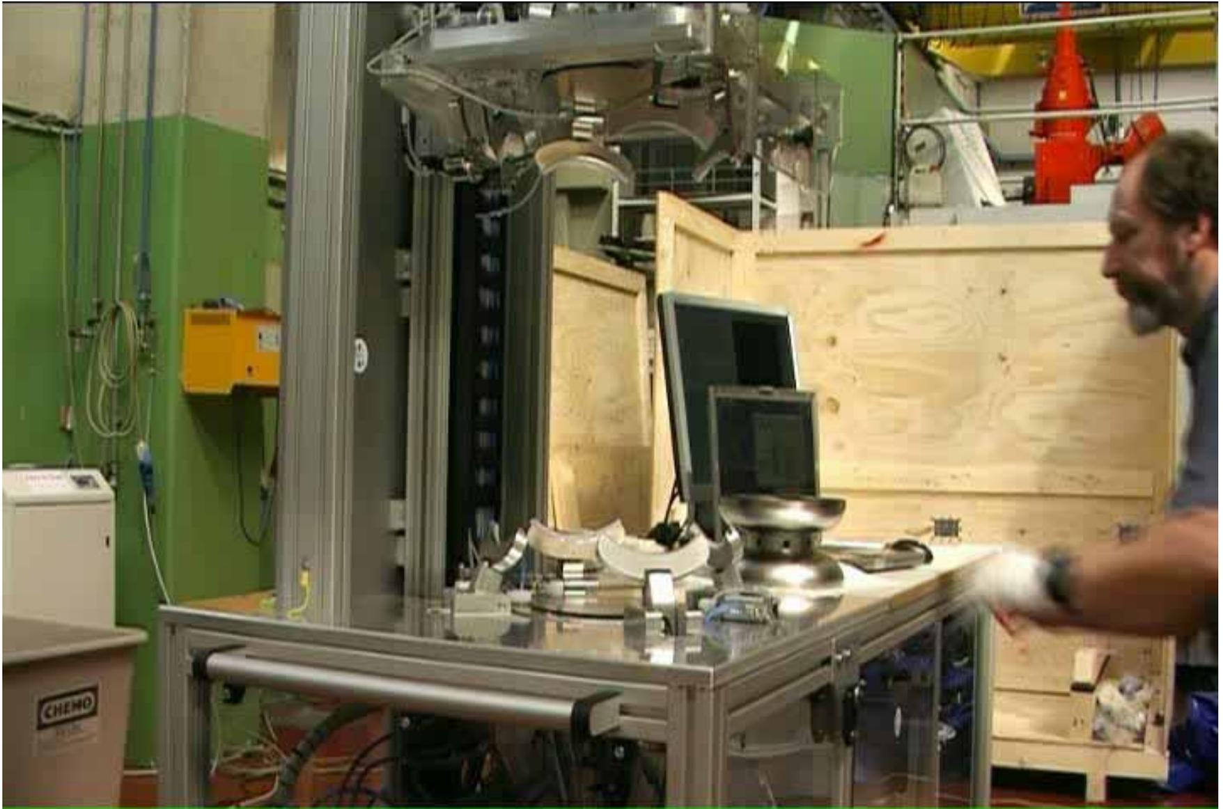
Equipment for RF measurement on half cells and dumb bells HAZEMEMA is developed at DESY for XFEL fabrication ([SRF2009, Poster THPP0071](#))
