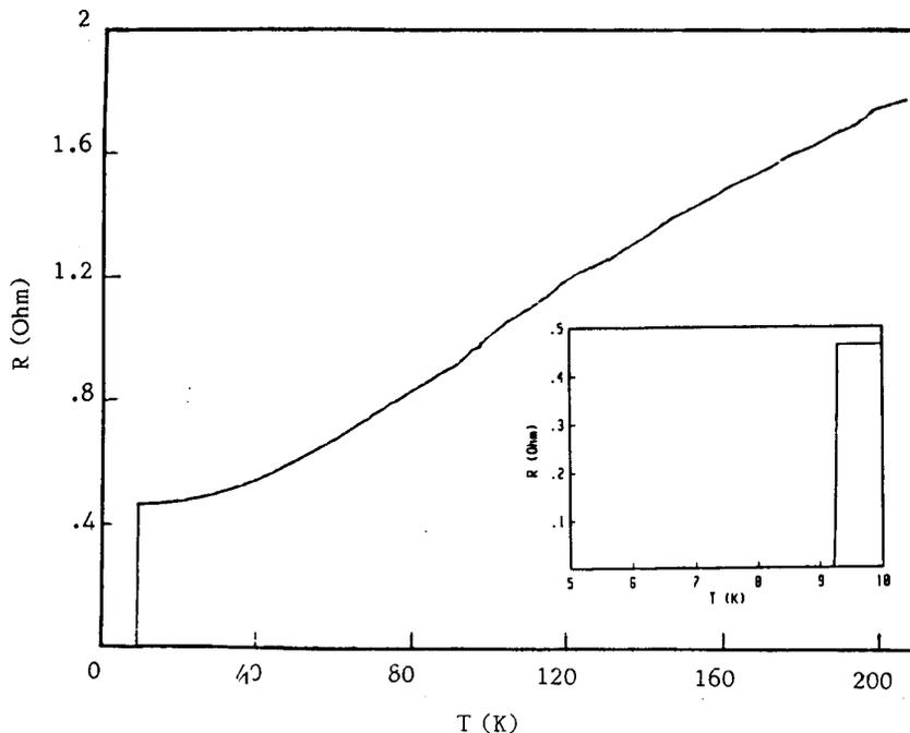
Fig. 4 - Resistance vs. temperature for Nb thin film.
