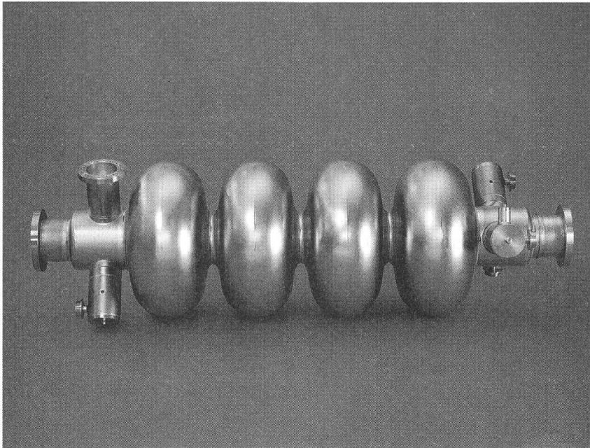
*Fig. 2 - One of the Nb cavities after welding.*
