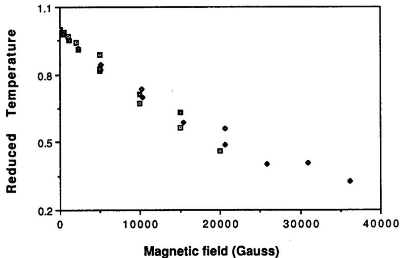
*Fig. 5 - Critical temperature vs. magnetic field for Nb thin film.*
