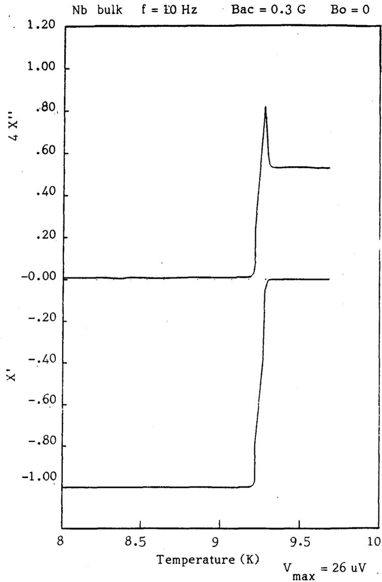
*Fig. 6 - Real and imaginary parts of susceptibility vs. temperature.*
