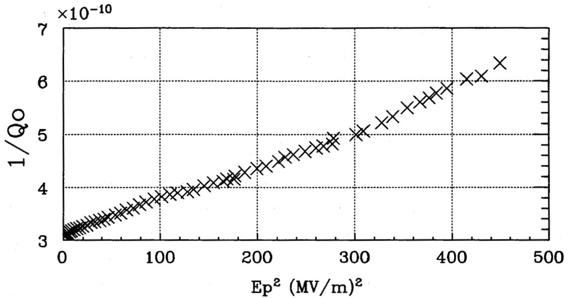
Fig.4 RF losses against square of peak surface field (Cavity #7b).
