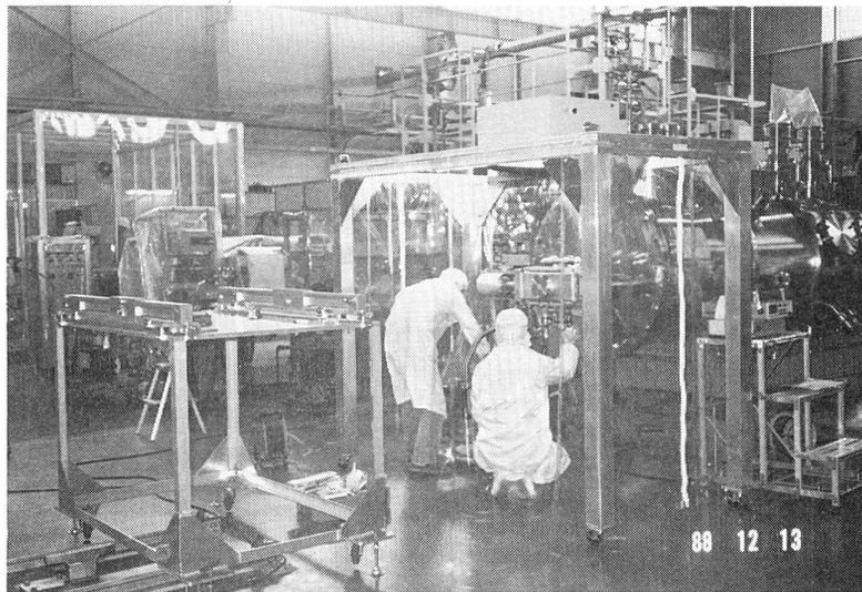
Fig.8 Portable plastic clean box for gate valve assembling.
