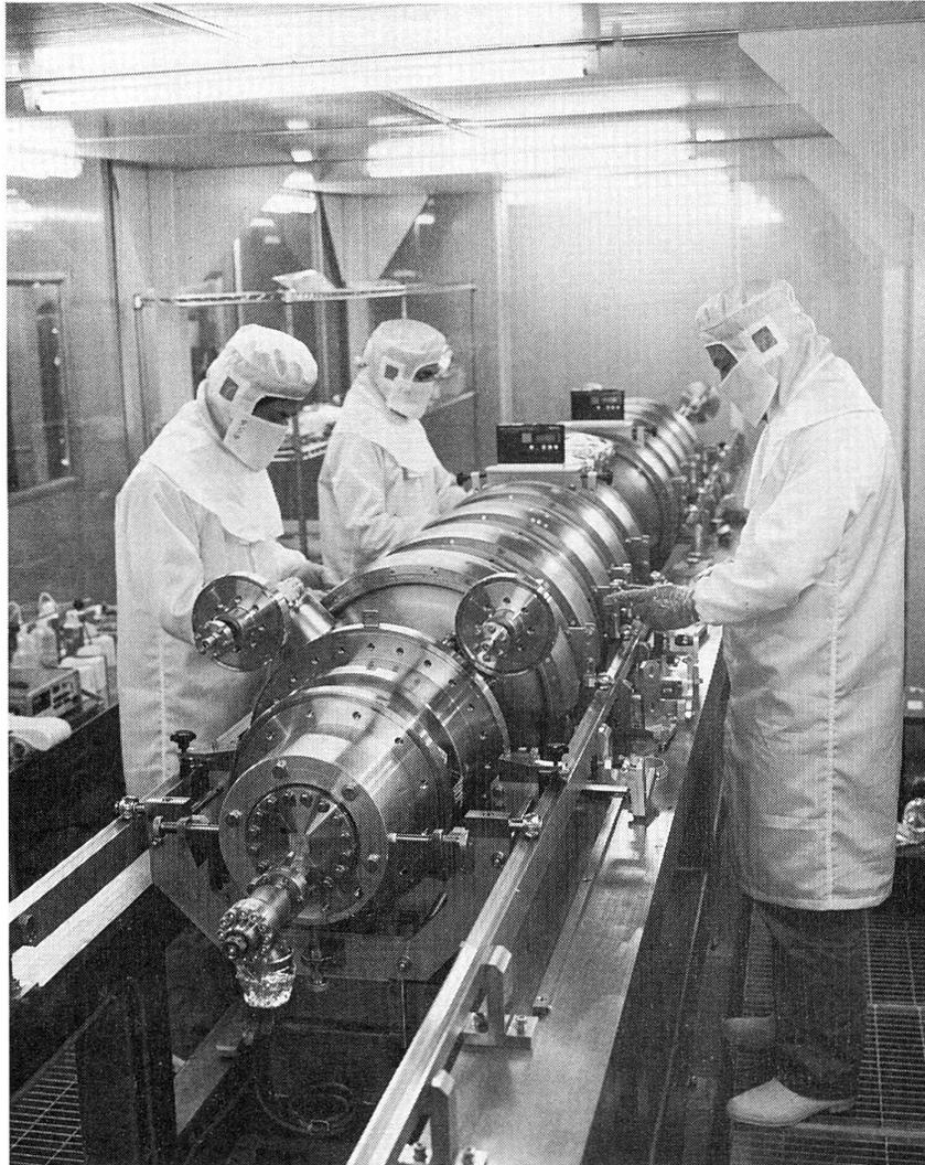
Fig.6 Cavity assembling in the clean room.
