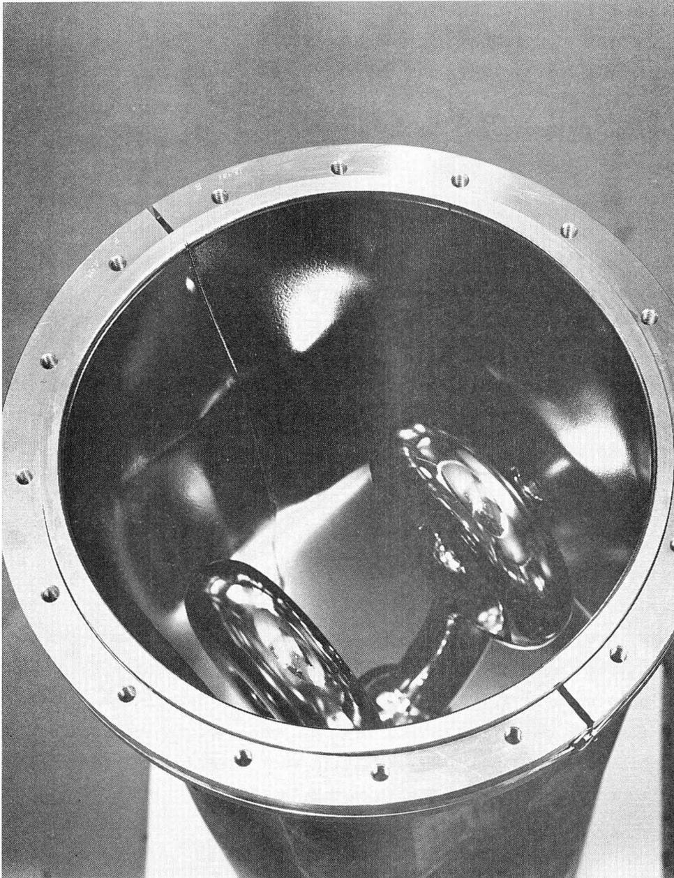
Figure 2 - Interior of an I3 type resonant cavity prior to final assembly.
