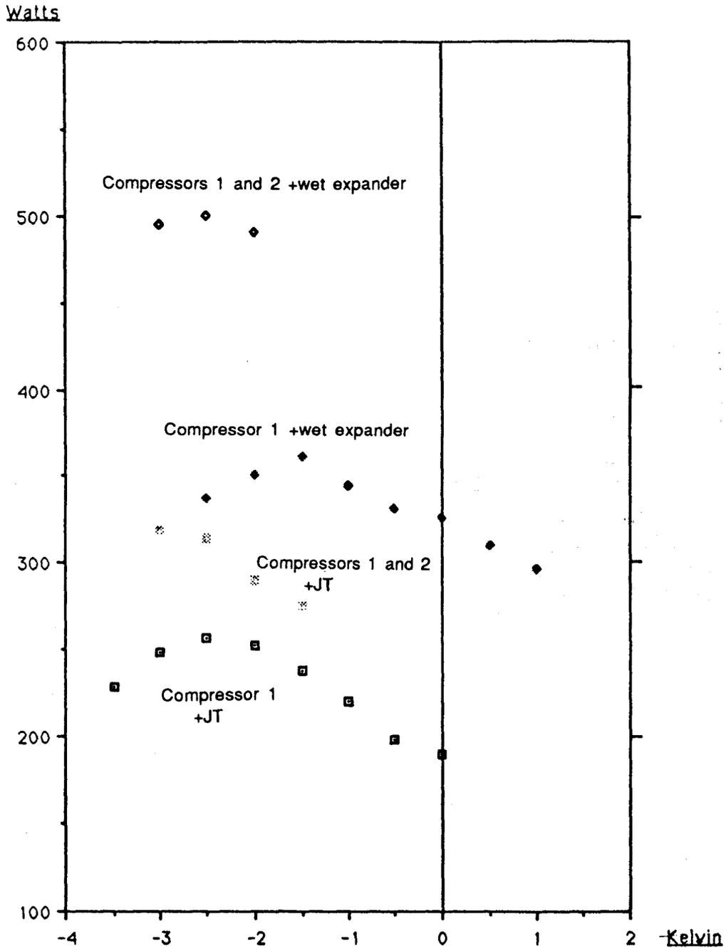
**Figure 3** Power at 4 K delivered by the refrigerator. The abscissa represent the temperature of the cold turbine outlet (0 is the initial setting). Absolute values of the temperatures are unknown.
