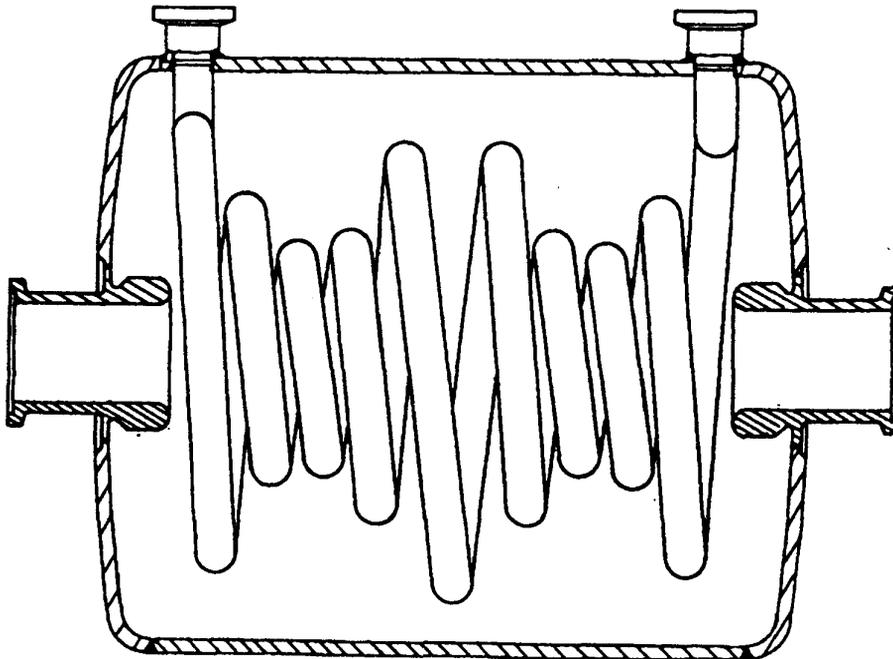
**Figure 1** Sketch of the  $\lambda$  resonator. The overall length is 33 cm. The RF magnetic field on the helix surface is maximum at the welds joining helix to can and also at the middle of the helix.
