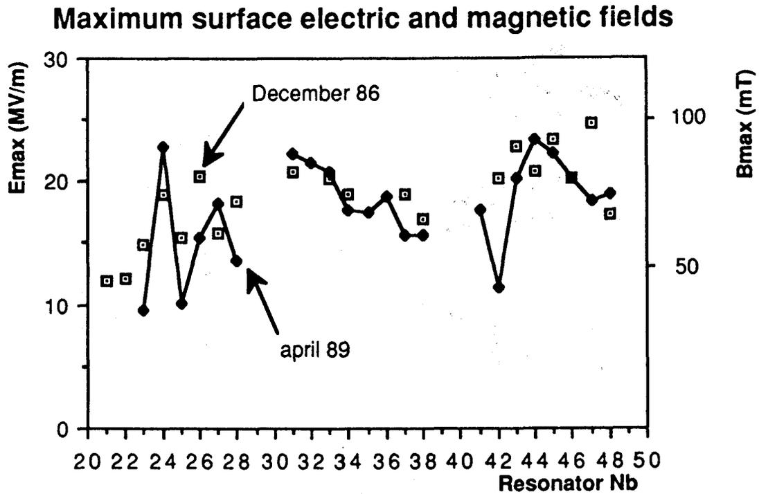
**Figure 5** Comparison of the maximum electric and magnetic surface fields measured with a  $^{12}\text{C}^{6+}$  beam in december 1986 (squares) and with an  $^{16}\text{O}^{8+}$  beam in april 1989 (solid line) for the resonators of the first leg of the machine. Resonators are identified on the horizontal axis according to their position (in december 1986) in the  $N^{\text{th}}$  cryostat (from N1 to N8). Data for the first high energy rebuncher (resonator #11) are not given.
