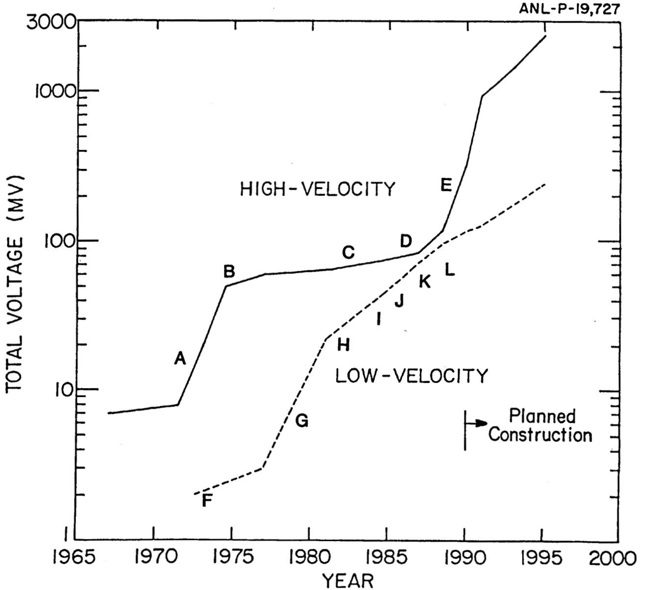
Figure 1. Integrated, accumulative voltage in test and/or operation of superconducting cavities with beam
