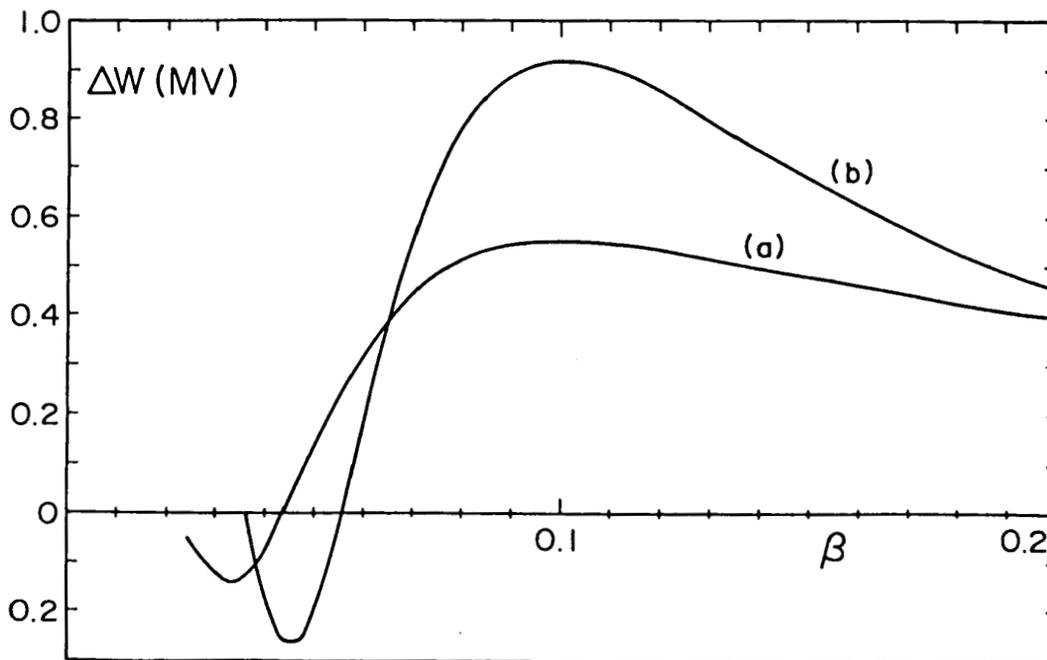
Figure 5. Voltage Gain as a Function of Velocity at a Peak Surface Field of 16 MV/m for Two 150 MHz,  $\beta = 0.1$  Structures: (a) 2-gap Structure, (b) 3-gap Structure
