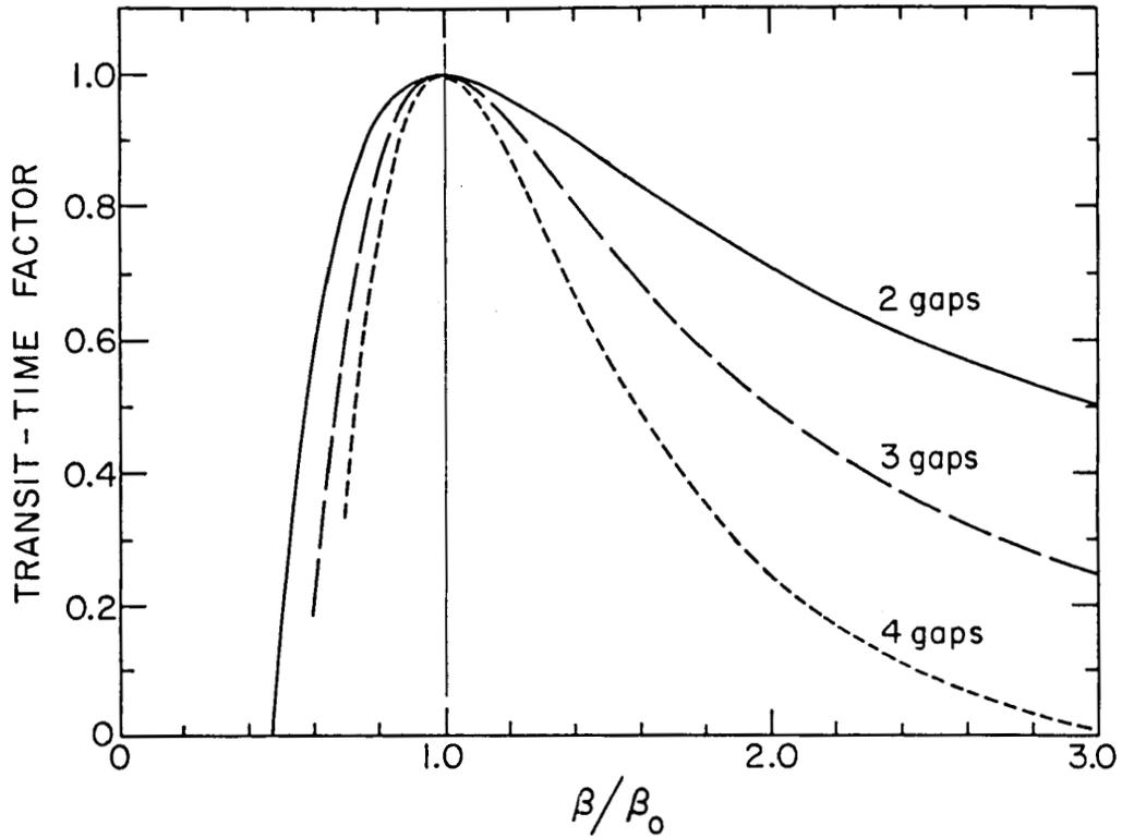
Figure 4. Transit Time Factor for 2, 3 and 4 Gap Structures
