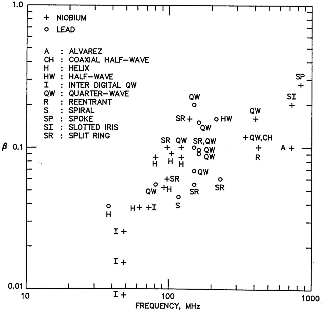
Figure 2: Superconducting Structures which have been Tested or are Under Development
