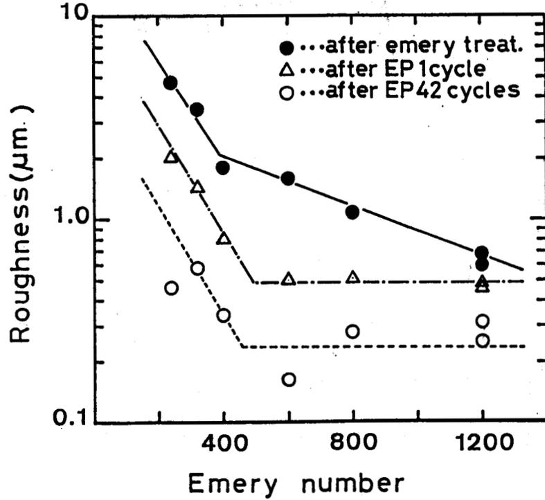
Figure 3: Effect of emery number to the surface roughness; after mechanically finished with various emery papers, and after subsequent electropolishing (1 cycle = 2 μm).
