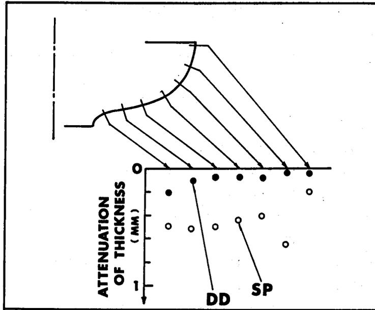
Figure 1: Comparison of the thickness attenuation between deep-drawing(DD) and spinning(SP); large attenuation causes the variety of thickness at the welding planes.
