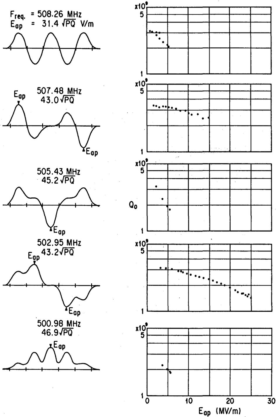
Figure 8: Passband modes measurements of #6a cavity.
