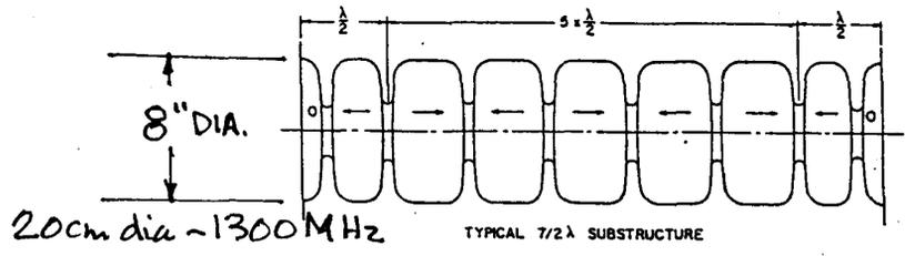
Fig. 5 Schematic of 20-foot accelerator structure and typical  $7/2\lambda$  sub-structures. The arrows show the relative direction of the axial electric field in the  $7/2\lambda$  sub-structure and in the individual cells. The cells which are joined by indium or lead seals are unexcited.
