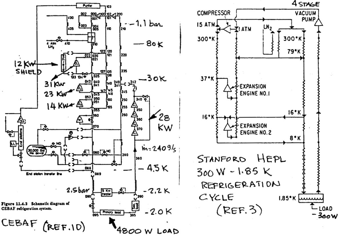
Figure 11.4.2 Schematic diagram of CEBAF refrigeration system.
