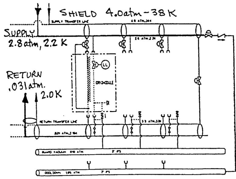
CEBAF Figure 11: Linac Transfer Line Schematic (REF. 10)
