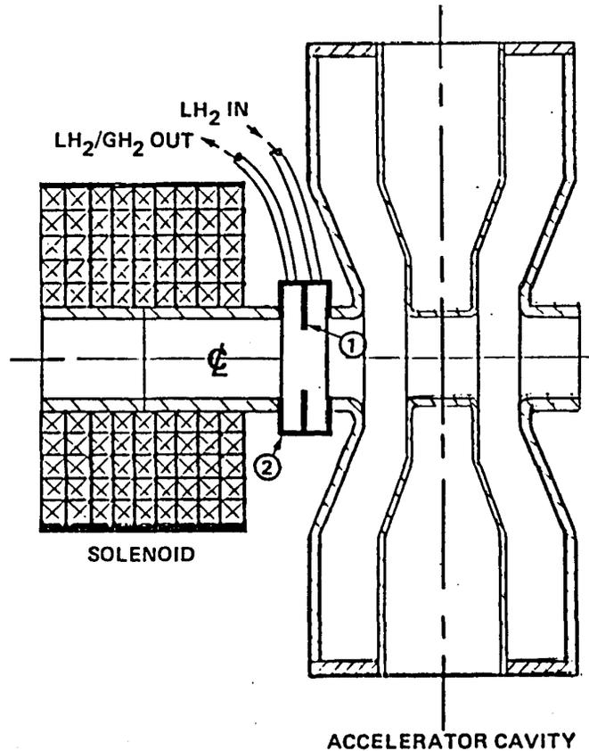
Figure 5. Conceptual focussing arrangement of a superconducting solenoid, beam block (1) to reduce beam impingement, and thermal isolator (2).
