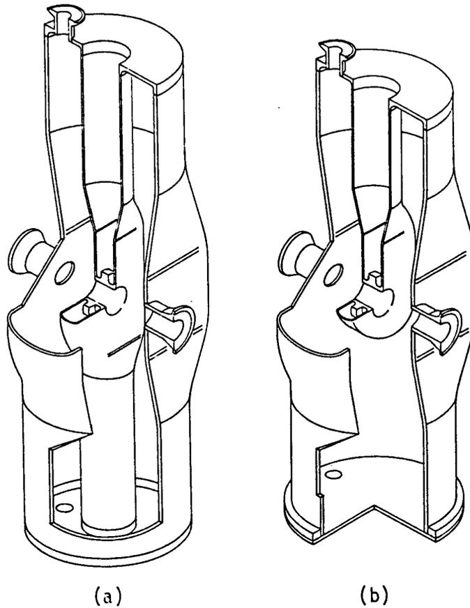
Figure 3. Conceptual design of (a) a coaxial half-wave resonator and (b) a coaxial quarter-wave resonator of frequency 352 MHz and particle velocity 0.12 c fabricated with high-conductivity sheet niobium.
