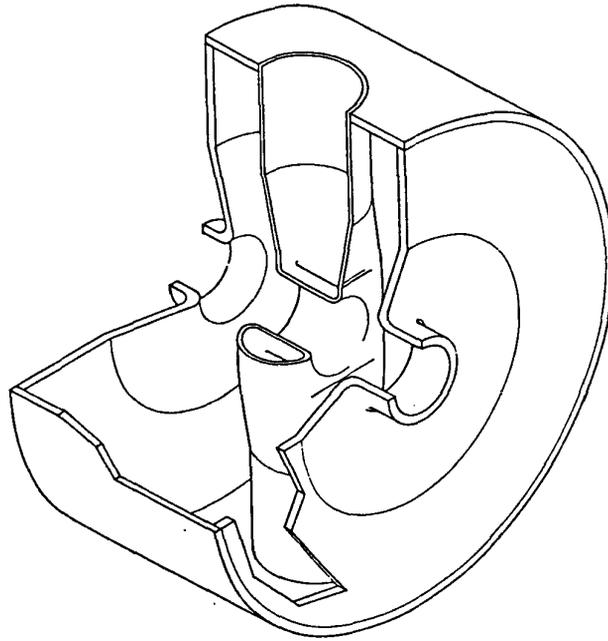
Figure 4. Conceptual design of a spoke resonator of frequency 850 MHz and particle velocity 0.28 c.
