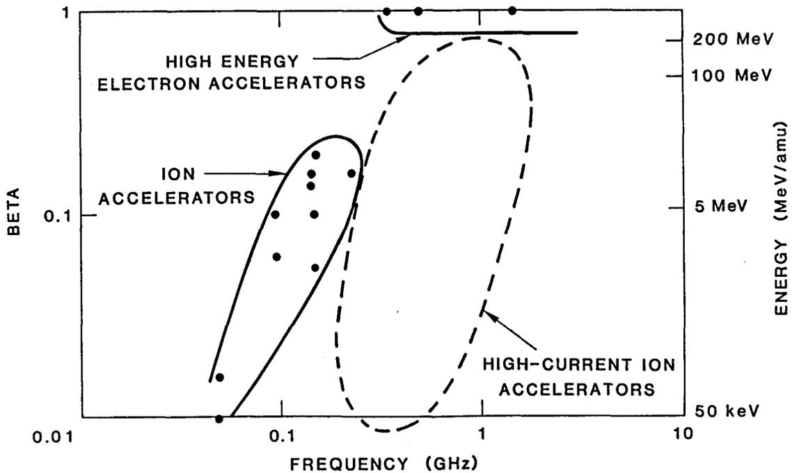
Figure 1. Phase velocity versus frequency of the superconducting cavities which are in use or at the advanced development stage.
