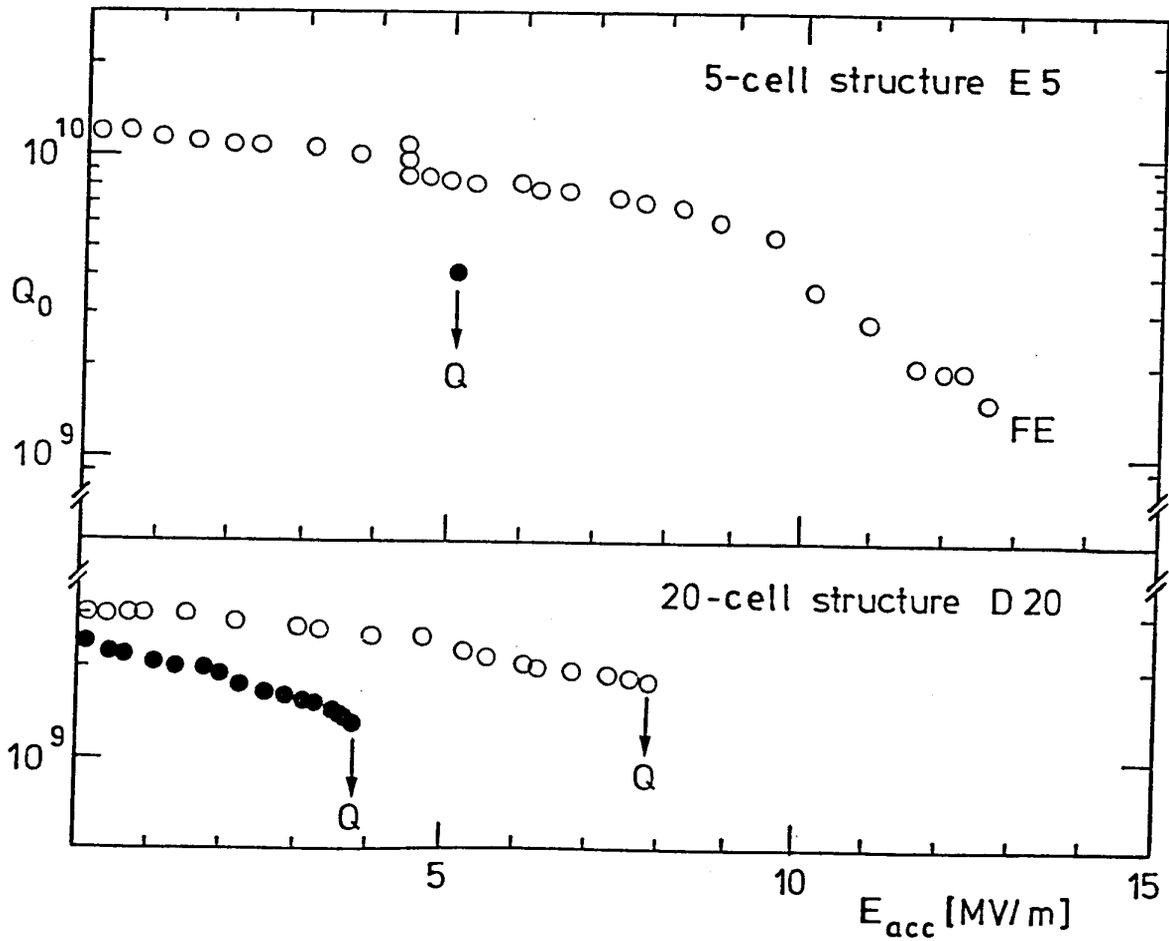
Fig. 2:  $Q_0$  ( $E_{acc}$ ) dependence of five cell, and 20 cell structure
