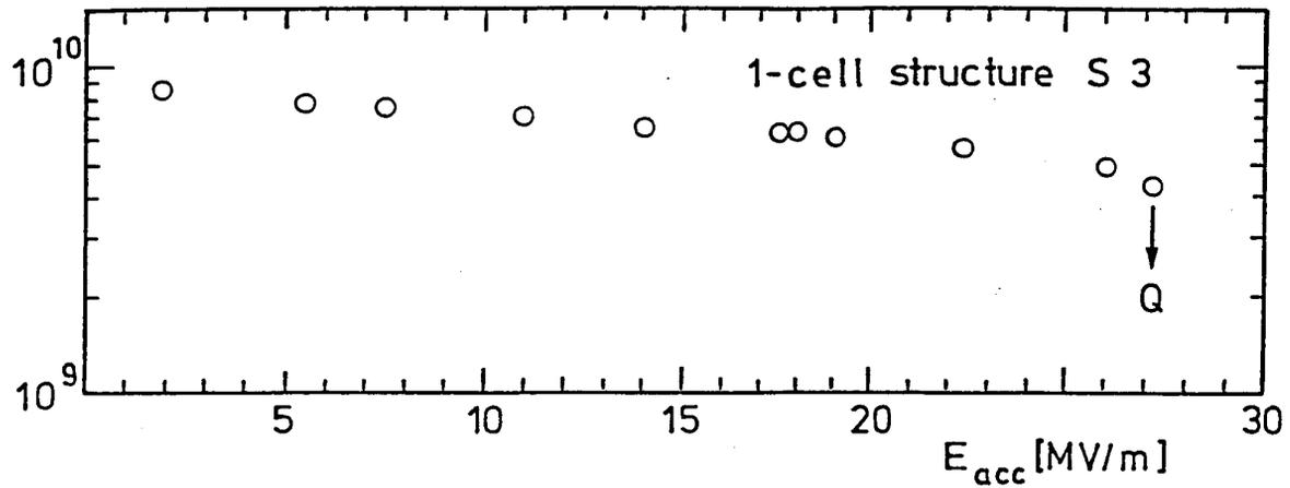
Fig. 1 :  $Q_0$  ( $E_{acc}$ ) dependence of single cell.
