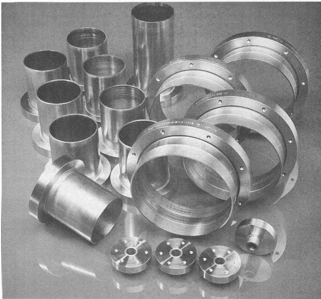
Fig. 10: Brazed niobium/stainless steel transition joints (cooperation with CERN/Geneva)
