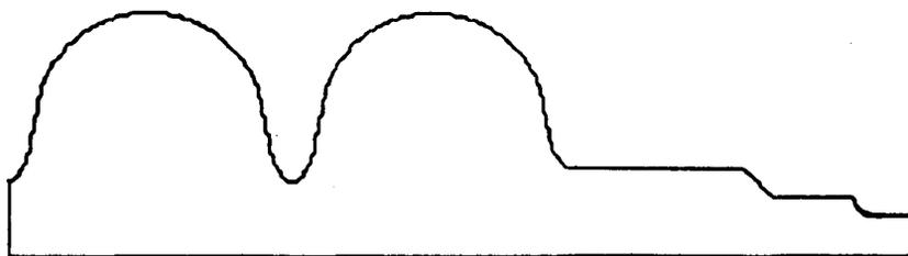
Figure 2. Cavity Shape used by URMEL
