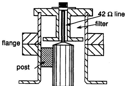
Fig. 3. Schematic of HOM Beamtube Coupler
