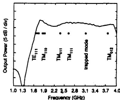
Fig. 4. Measured Response of HOM Coupler
