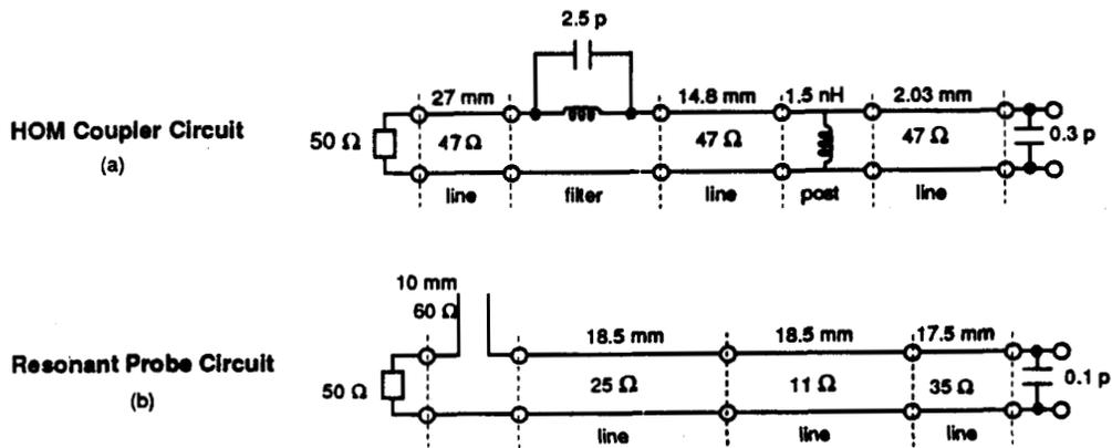
Figure 7. Equivalent Circuits for HOM Coupler and Probe.
