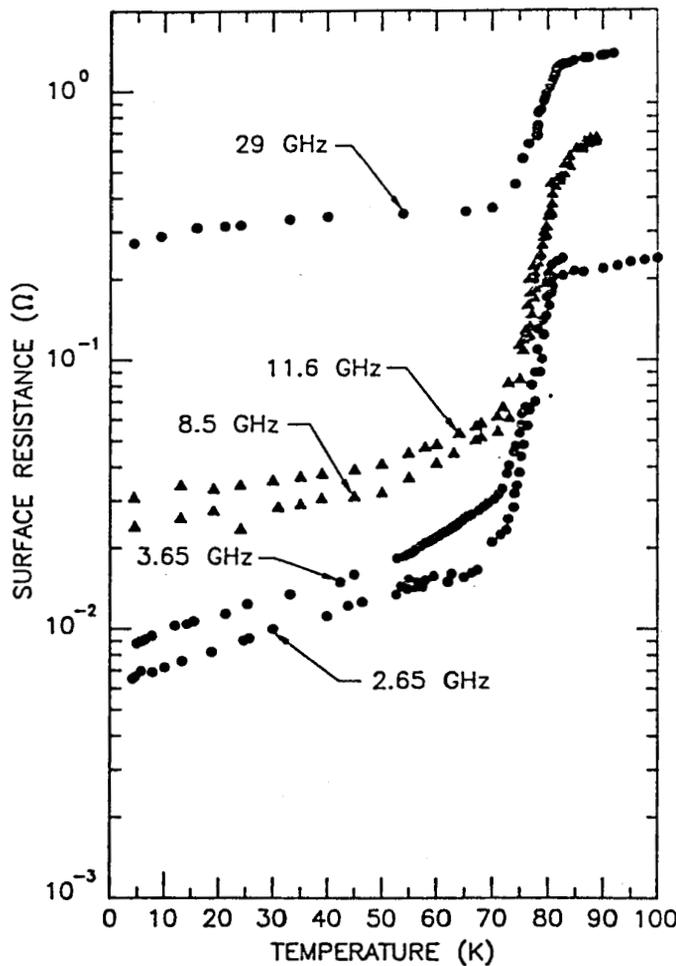
Figure 5. RF surface resistance versus temperature of BSCCO thick films on silver at low field ( $B_{rf} \leq 0.1$  G). Circles correspond to the 4336 samples; triangles correspond to the 2212 sample.
