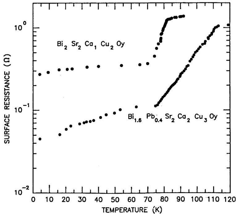
Figure 6. Comparison of rf surface resistance versus temperature at low field of bulk Pb-doped BSCCO versus BSCCO thick film on silver at 29.2 GHz.
