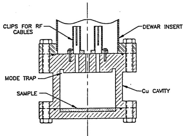
Figure 2. Generic TE cavity. The sample is the bottom surface of the cavity.
