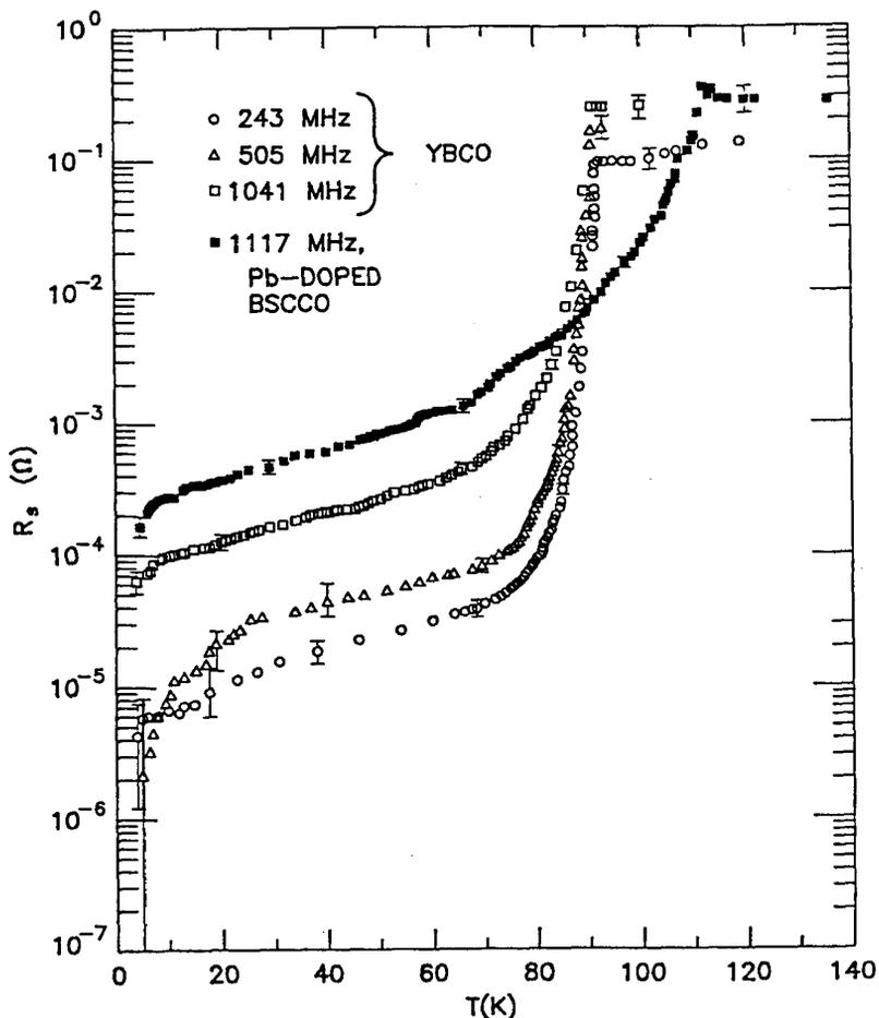
Figure 3. Surface resistance of bulk YBCO versus temperature at three frequencies and at low field ( $B_{rf} \lesssim 0.05$  G). Low-field data for a bulk Pb-doped BSCCO sample at 1.1 GHz is also shown.
