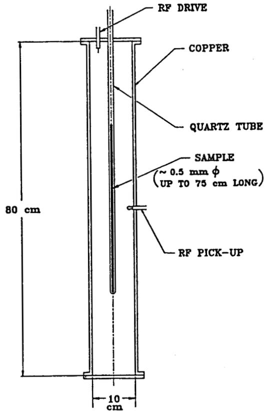
Figure 1. Generic TEM cavity. The sample is a rod which acts as a resonant coaxial line.
