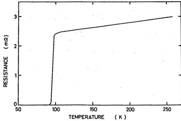
Fig.5 Temperature dependence of the DC resistance of a  $YBa_2Cu_3O_{7-x}$  bulk sample.
