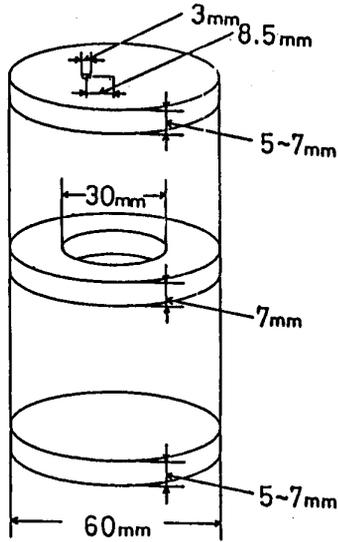
Fig.1 Assembly of a TE<sub>011</sub> mode cavity using YBa<sub>2</sub>Cu<sub>3</sub>O<sub>7-x</sub> disks and ring.
