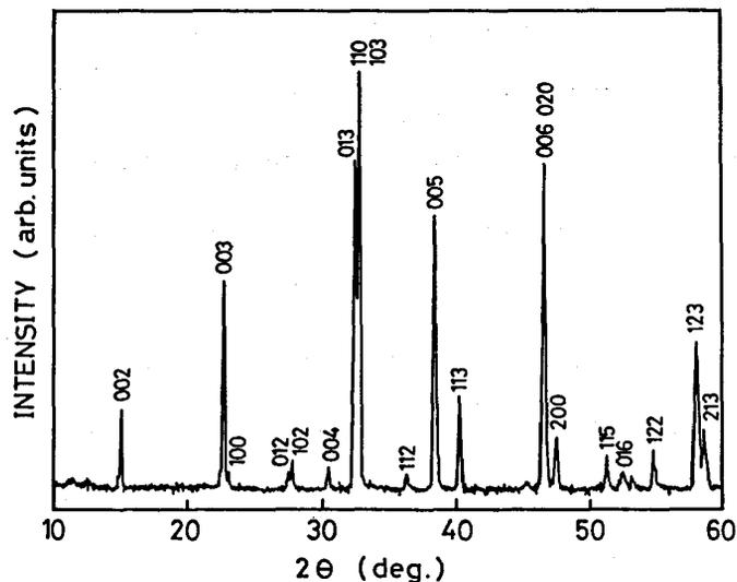
Fig.4 X-ray diffraction pattern for a  $YBa_2Cu_3O_{7-x}$  bulk sample.
