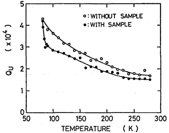
Fig.10 Temperature dependence of the unloaded quality factor of the cavity with or without the sample.
