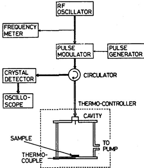
Fig.9 Schematic diagram of the quality factor measurements of the  $TM_{011}$  mode cavity with a  $YBa_2Cu_3O_{7-x}$  disk sample.
