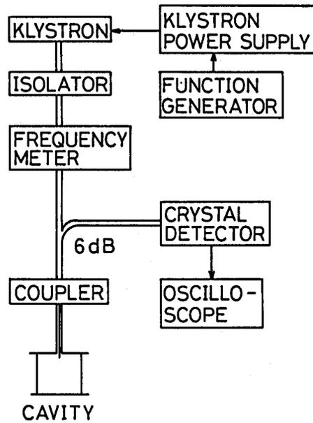
Fig.3 Schematic diagram of microwave measuring system.
