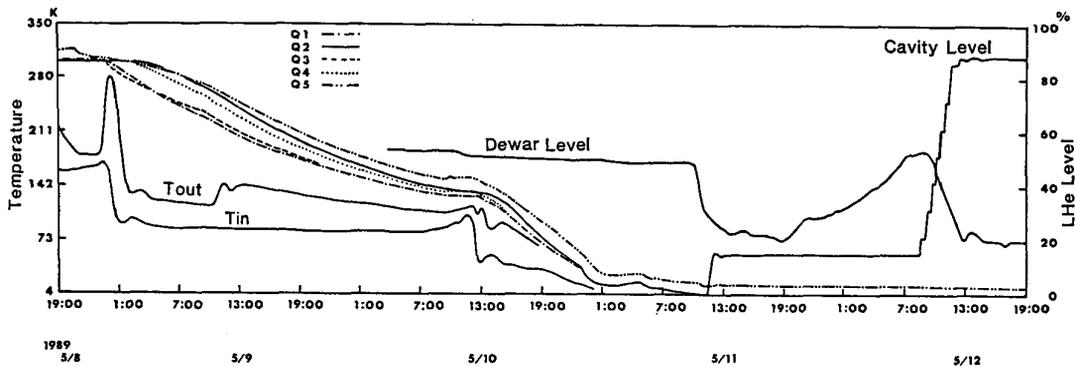
**Figure 7** Cool down curves of SCC cryostat.
