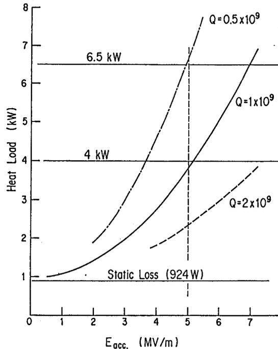
Figure 3 Total heat load of the SCC (32 x 5-cell) cryogenic system as a function of accelerating field  $E_{acc}$ .
