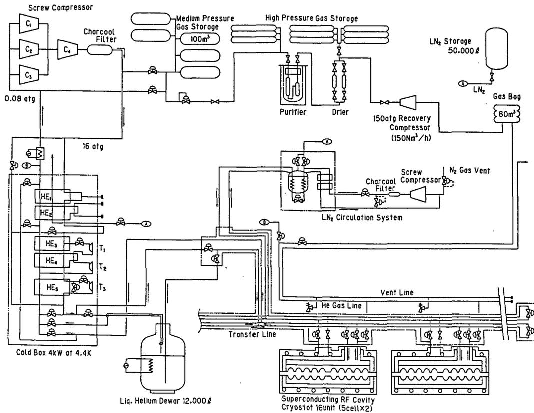
Figure 1 Schematic flow diagram of TRISTAN SCC cryogenic system.
