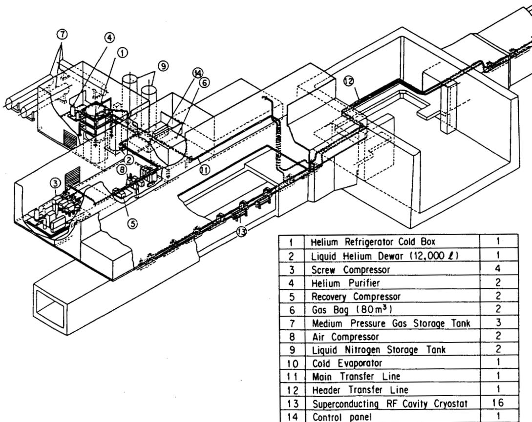
Figure 2 An isometric showing of cryogenic equipments layout.
