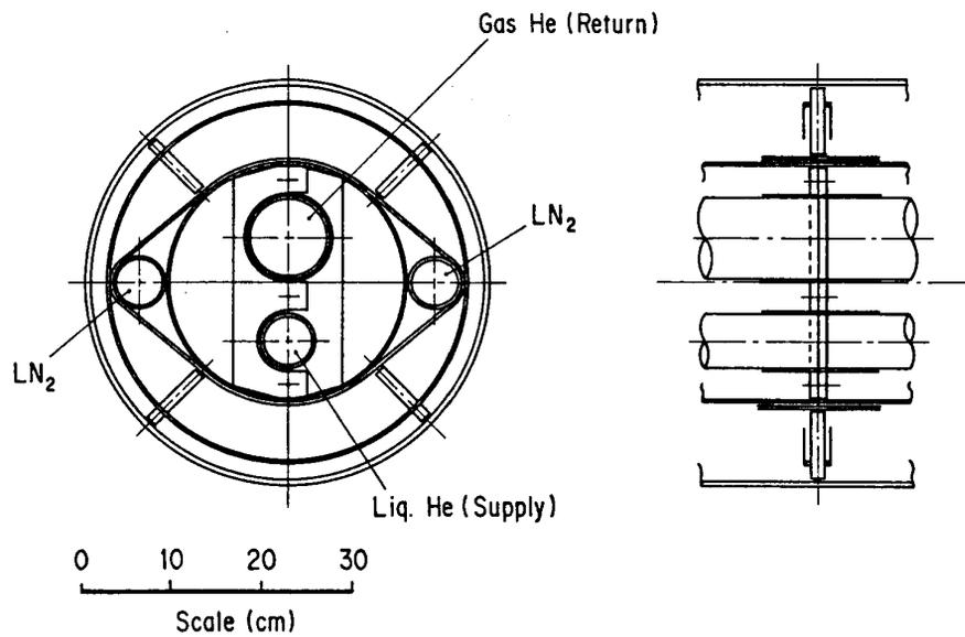
Figure 5 Cryogenic transfer line.
