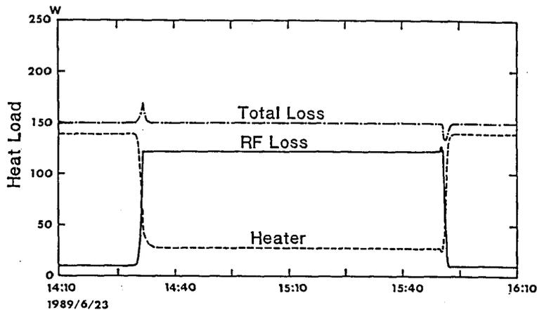
Figure 9 RF loss, compensation heater and total heat load curves.
