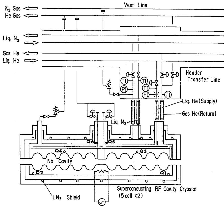
Figure 4 Schematic drawing of SCC. The location of temperature sensors are shown as small circles.
