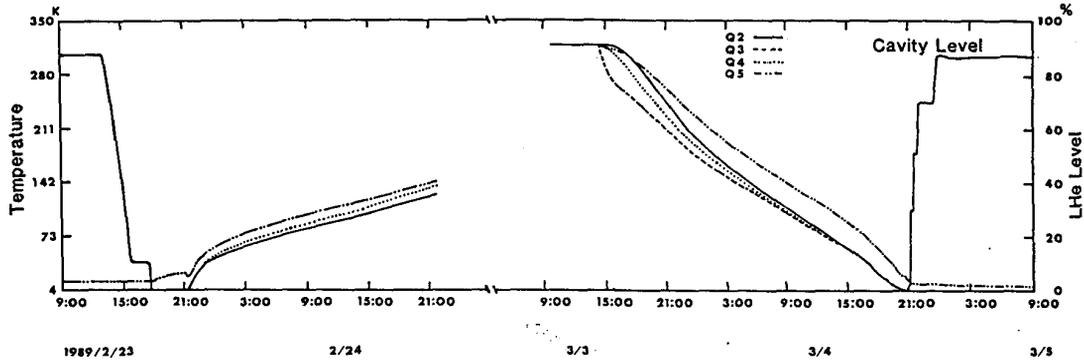
Figure 8 Warm up and cool down curves of one SCC cryostat.
