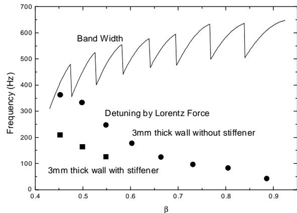
Fig. 14 Frequency shift by Lorentz force (given in absolute values) and the cavity band width
