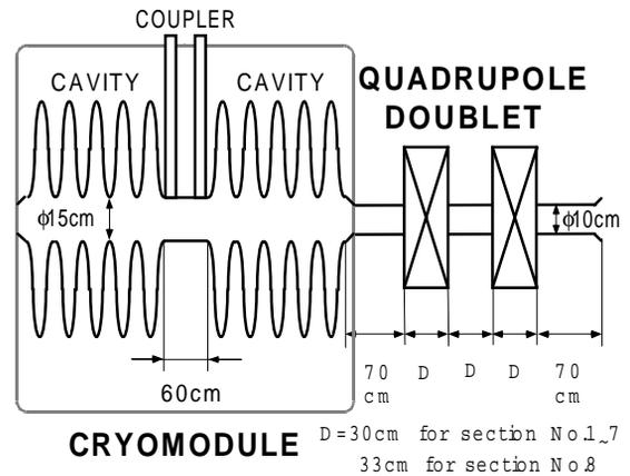
Fig. 4 Schematic view of the beam line
