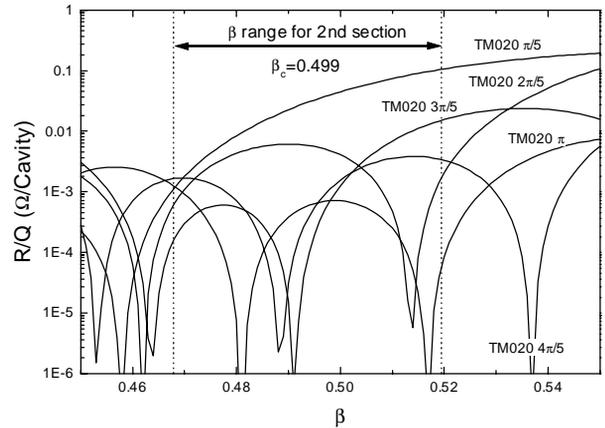
Fig. 11 R/Q values of the TM020 modes as a function of  $\beta$  for the 2nd cavity
