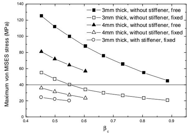
Fig. 12 Maximum von MISES stress of the cavity against static vacuum load
