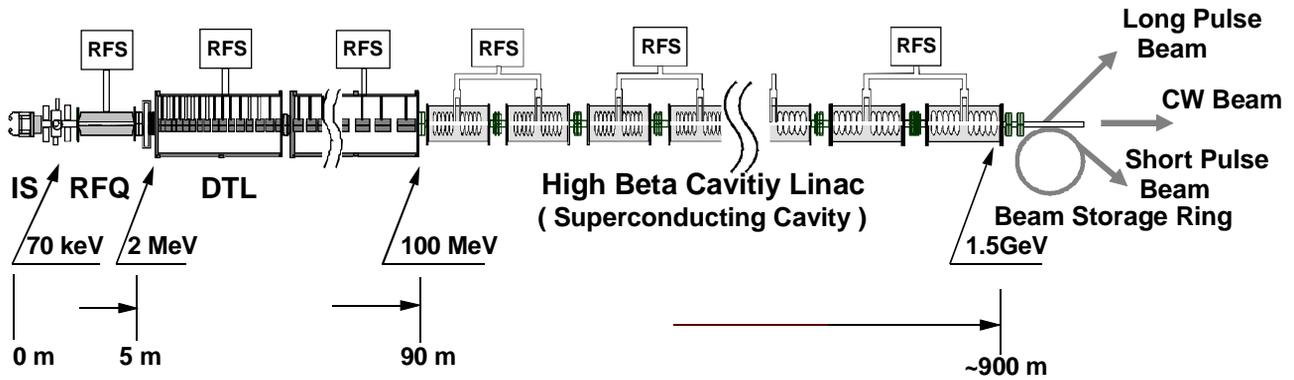
Fig. 2 Conceptual layout of the NSP linac
