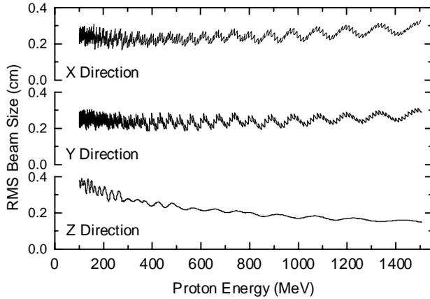
Fig. 7 The rms beam size obtained by the beam simulation
