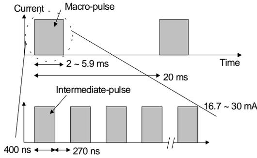
Fig. 3 Pulse structure for the neutron Scattering facility
