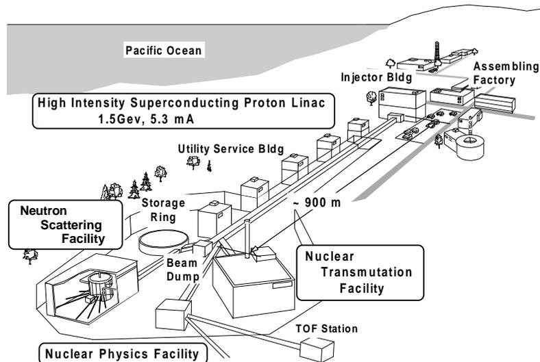
Fig. 1 Facility layout of the Neutron Science Project (NSP)
