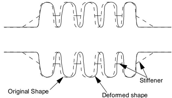
Fig. 13 Lowest vibration mode (80Hz) for the  $\beta_c=0.499$  cavity of 3 mm thick wall with stiffener
