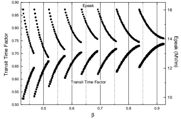
Fig. 6 Transit time factor and  $E_{\text{peak}}$  as a function of the reference particle  $\beta$
