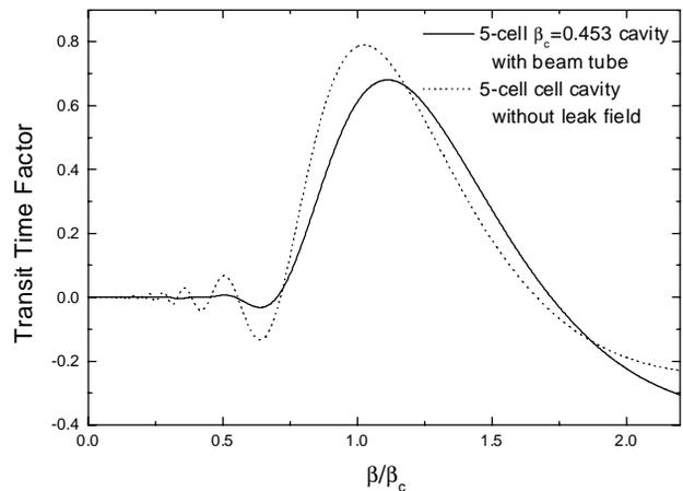
Fig. 10 Transit time factor for 5-cell  $\beta_c = 0.453$  cavity as a function of  $\beta/\beta_c$
