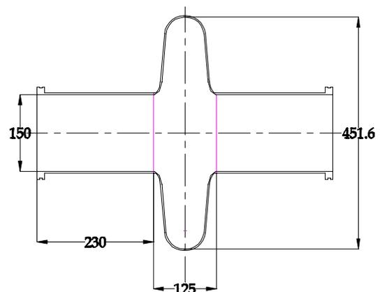
Fig. 3 Cross sectional view of the single cell cavity of  $\beta=0.5$
