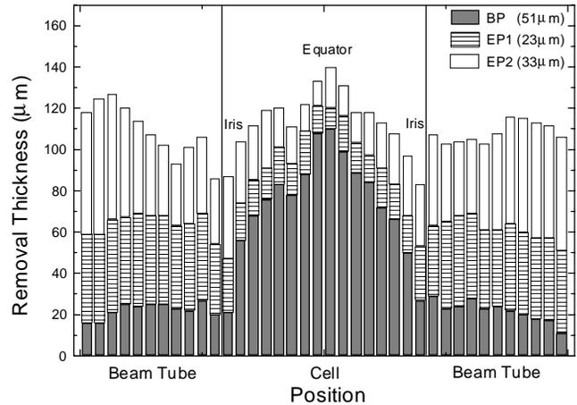
Fig. 4 Distribution of removal thickness in the barrel polishing (BP) and the electropolishing (EP1, 2)
