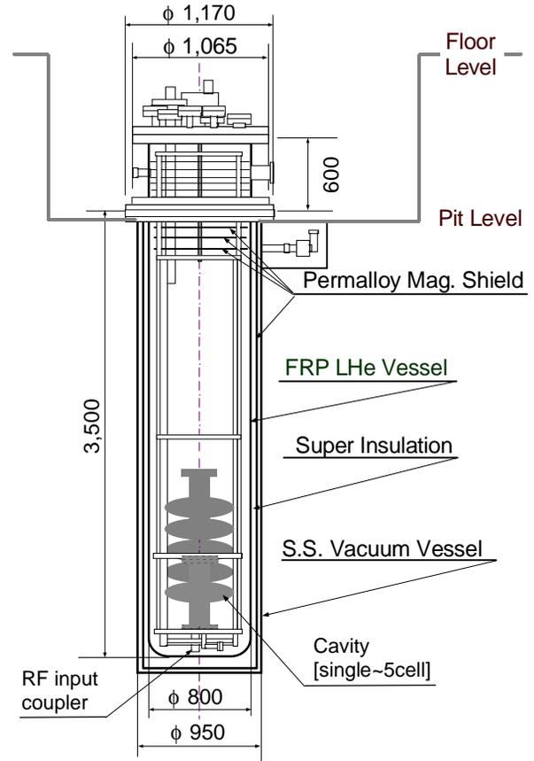
Fig. 2 Schematic view of the cryostat
