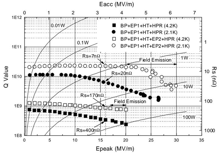
Fig. 5 Q values of the  $\beta=0.5$  single cell cavity as a function of peak surface electric field ( $E_{\text{peak}}$ )
