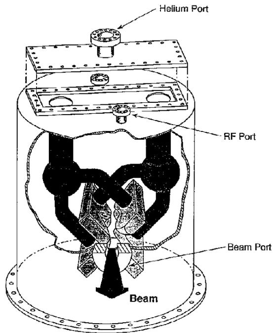
Figure 2. Schematic of SUNY prototype
