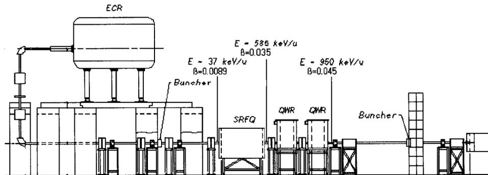
Figure 6 The schematic layout of PIAVE.
