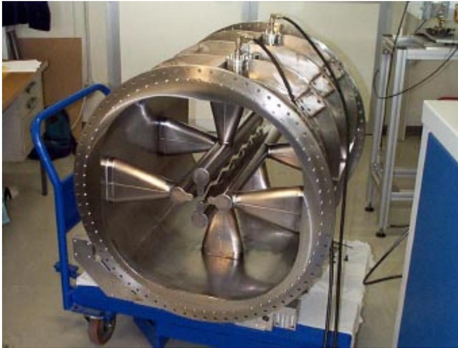
Figure 8. View of the stainless steel model of the Legnaro SRFQ resonator number 2
