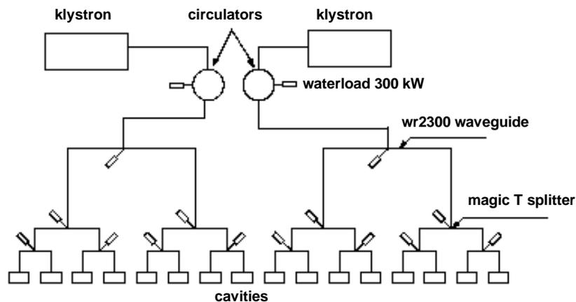
Fig. 3 Layout of twin RF units sharing common klystron supply
