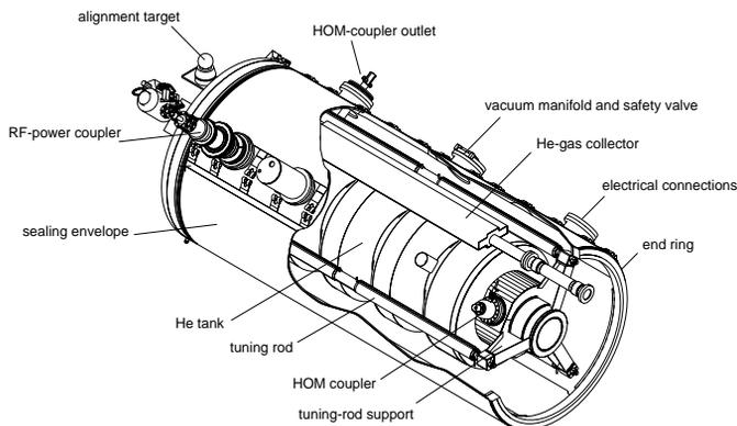
Fig. 1 LEP superconducting cavity
