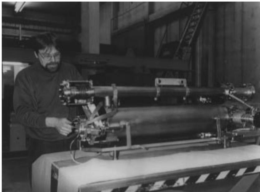
Fig. 7 A 9-cell cavity is welded into the LHe tank (lower cylinder). The cold end of the input coupler is visible at the right end, the tuner is assembled at the left end, the LHe line is shown on top of the structure.
