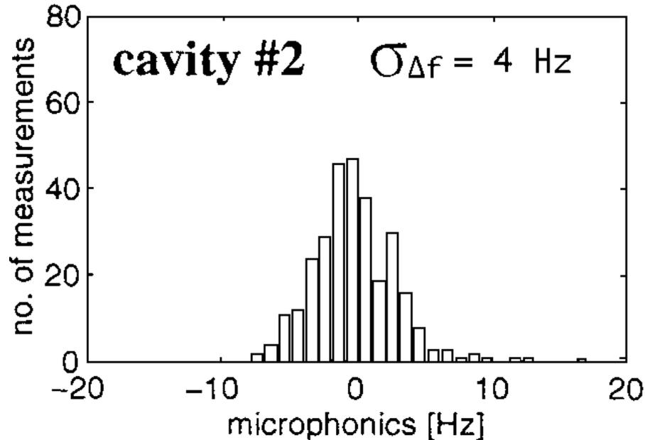
Fig. 13 Result of the search for microphonics: the resonance frequency of a cavity in the module is measured and statistically evaluated. No microphonics is present because the frequencies are centred around the nominal value.
