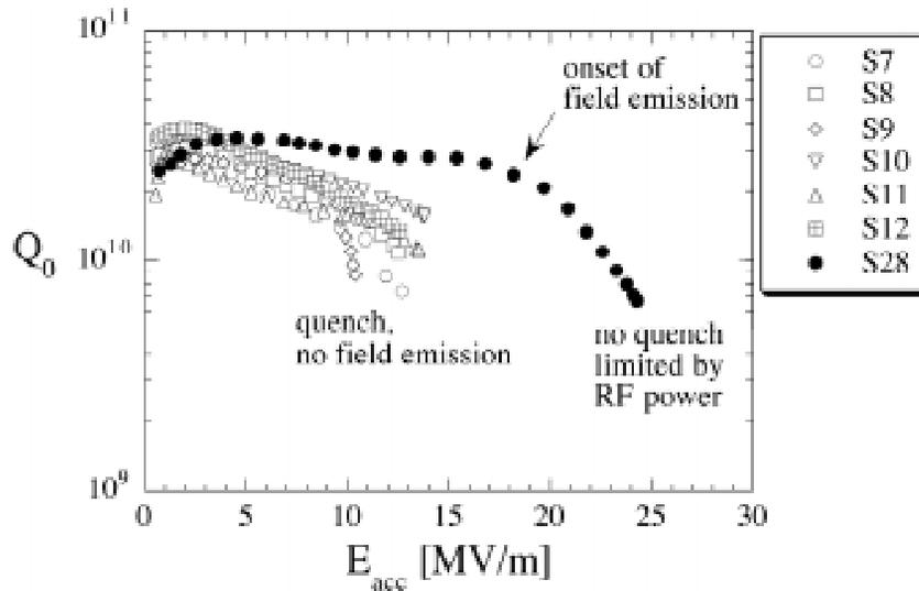
Fig. 4 Performance of 6 cavities from one vendor: decrease of the Q value at low gradients (but no field emission) and early thermal breakdown between  $E_{acc}$  10 to 14 MV/m. The defects were localised at the equatorial welding and could be traced back to improper cleaning and not optimised welding parameters. One more cavity was fabricated with improved fabrication conditions and showed excellent performance (S28).
