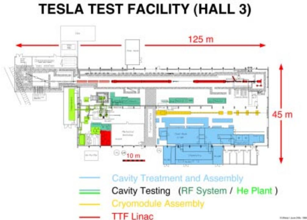
Fig. 1 Experimental hall of the TESLA Test Facility (TTF): chemical processing, clean room assembly and test preparation at the lower right; vertical and horizontal test areas at the lower left; linac installation in the upper half.
