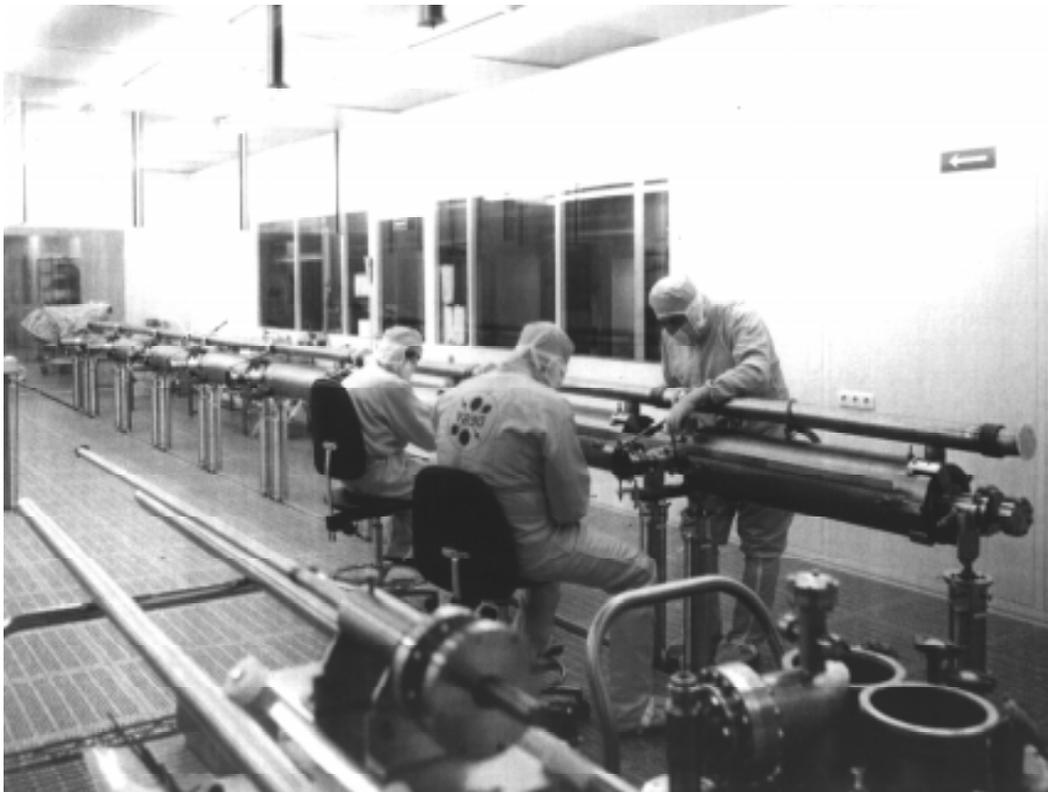
Fig. 8 Assembly of a string of 8 9-cell cavities and one quadrupole during handling in the clean room.
