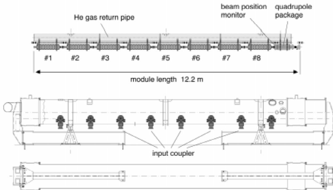
Fig. 10 Longitudinal cut through one module (8 cavities, one quadrupole) of the TTF cryostat.
