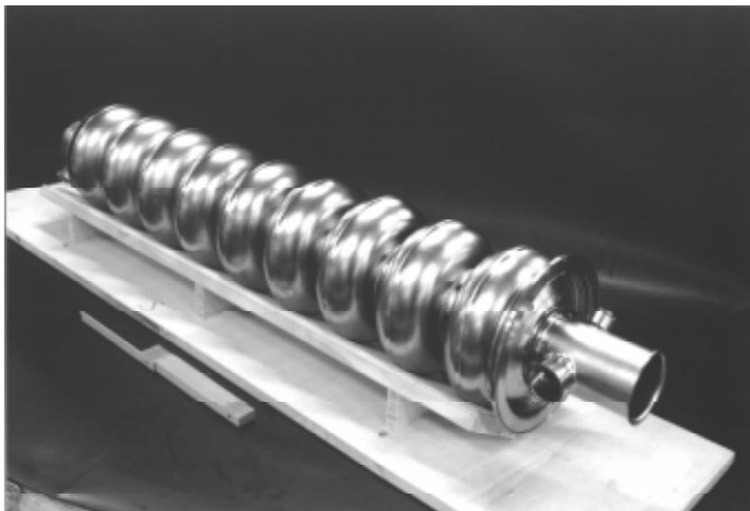
Fig. 2 9-cell TTF cavity. On the right beam pipe the port for the input coupler (front side) and the HOM coupler (back side) can be seen.
