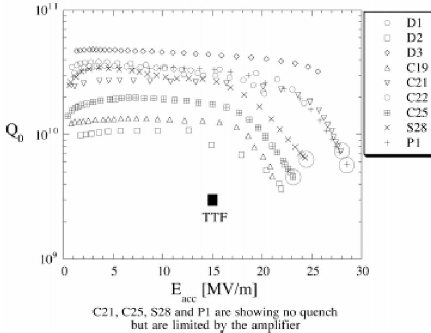
Fig. 3 Performance of “good” cavities in the vertical measurement. Four cavities (C21, C25, S28, P1) were limited by available RF power. The typical decrease of the Q value at high gradients is due to field emission.
