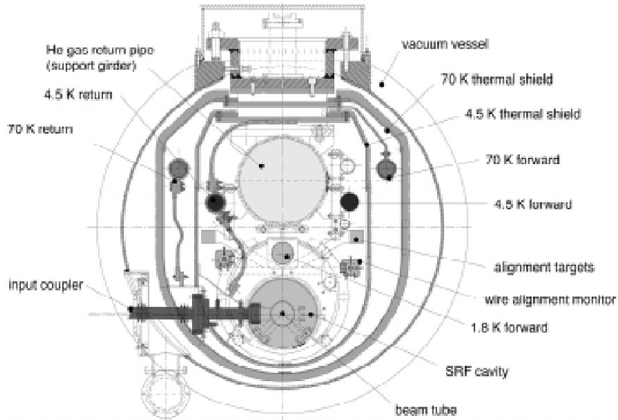
Fig. 9 Cross section of the cryostat for TTF
