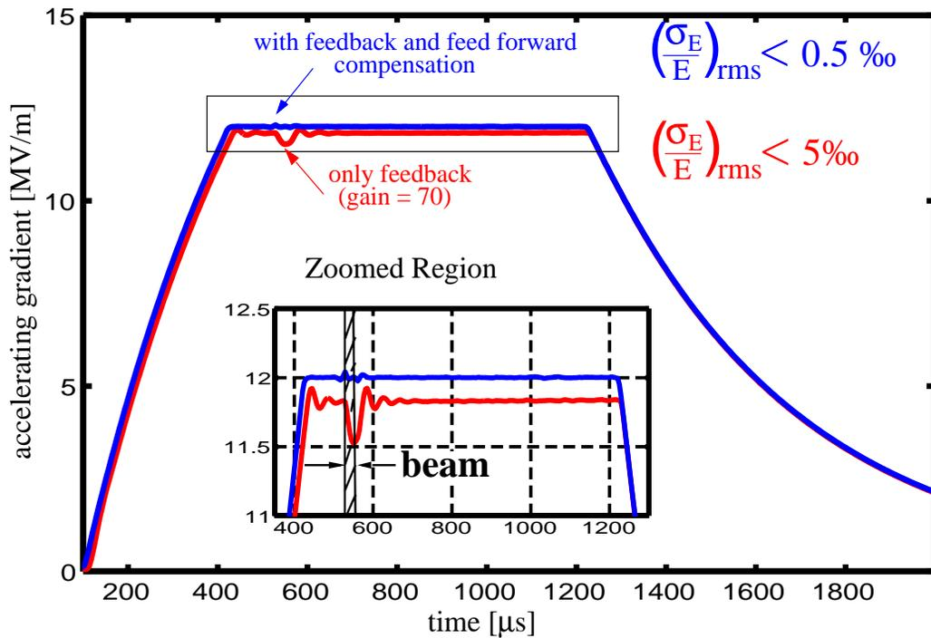
Fig. 12 Cavity voltage during pulsed operation with beam. The fluctuation of the cavity voltage is smaller 5 ‰ with feed back and reduced to smaller 0.5‰ with additional feed forward compensation.
