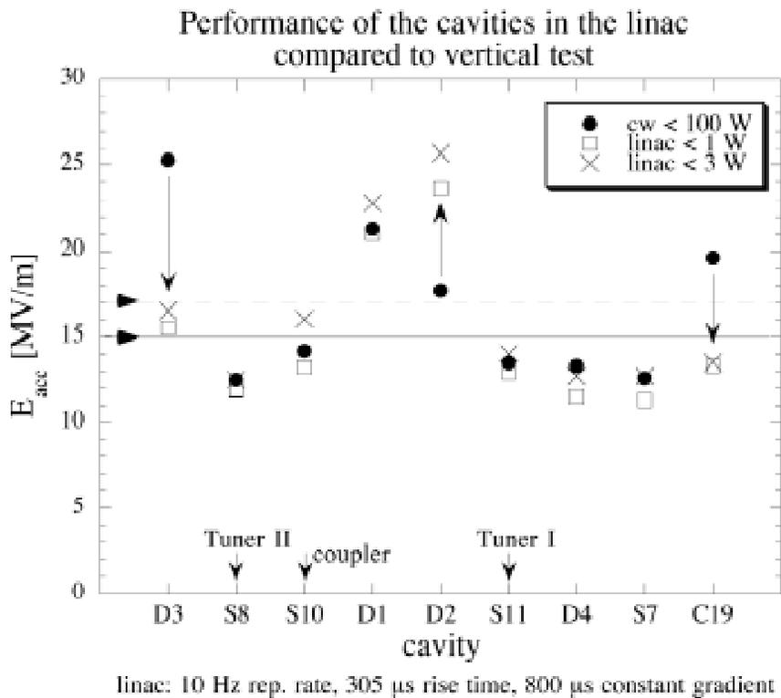
Fig. 11 Performance of the cavities in vertical tests (dark circle) and in the linac module (cross, open square). The gradient  $E_{\text{acc}}$  is noted just below thermal breakdown or at the onset of field emission. The cavity D2 upgraded in the linac operation because the time constant of the thermal breakdown is longer than the linac RF pulse. Cavities D3 and C19 degraded because of enhanced field emission.
