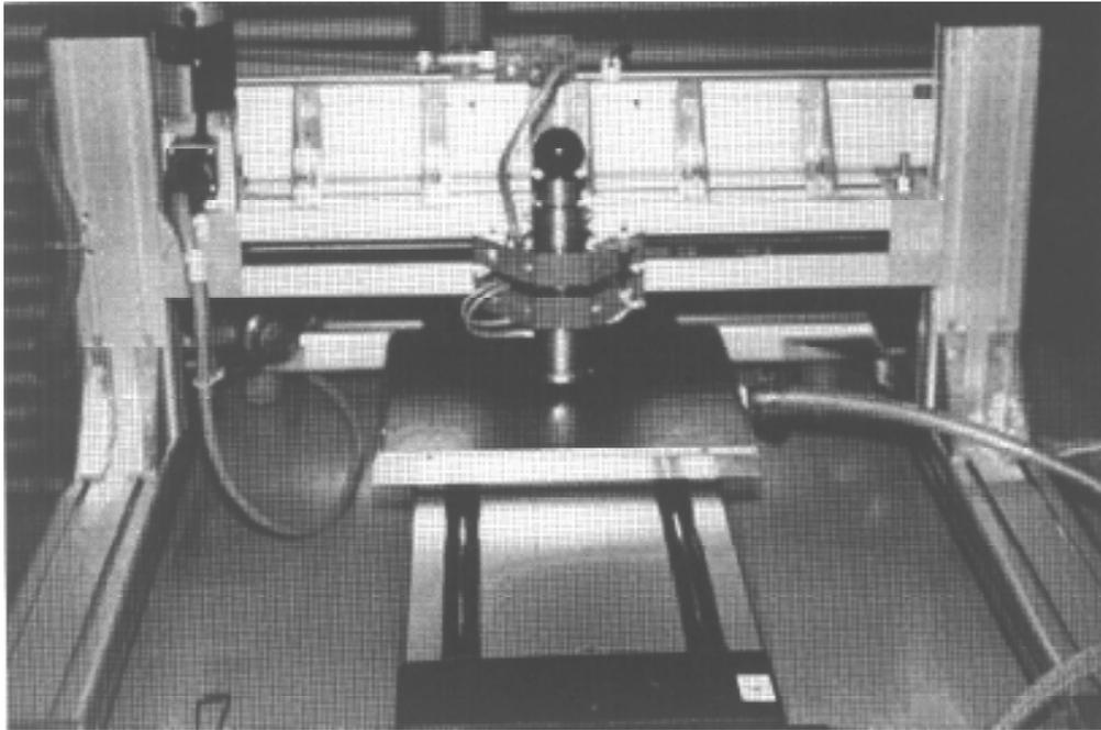
Fig. 14 Eddy current scanning apparatus for quality control of Nb sheets.
