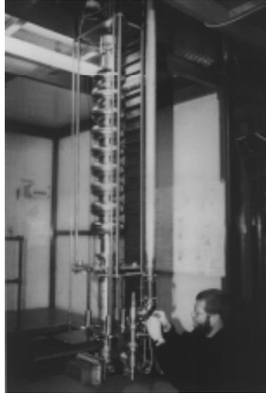
Fig. 6 Vertical test stand for acceptance test of the 9-cell cavities. The rectangular waveguide parallel to the cavity will transport RF power for high power pulse processing (HPP)
