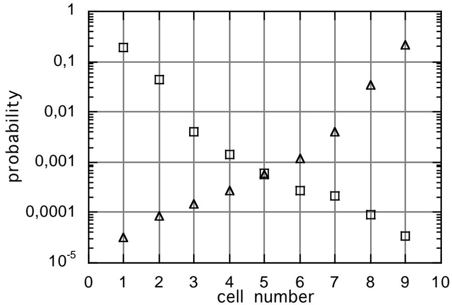
Fig. 7: Probability that a photon enters the beam pipe in logarithmic scale versus cell number. During one measurement the position of the solar cell and the black box where exchanged from the left beam pipe to the right beam pipe. Thus we measured two curves.
