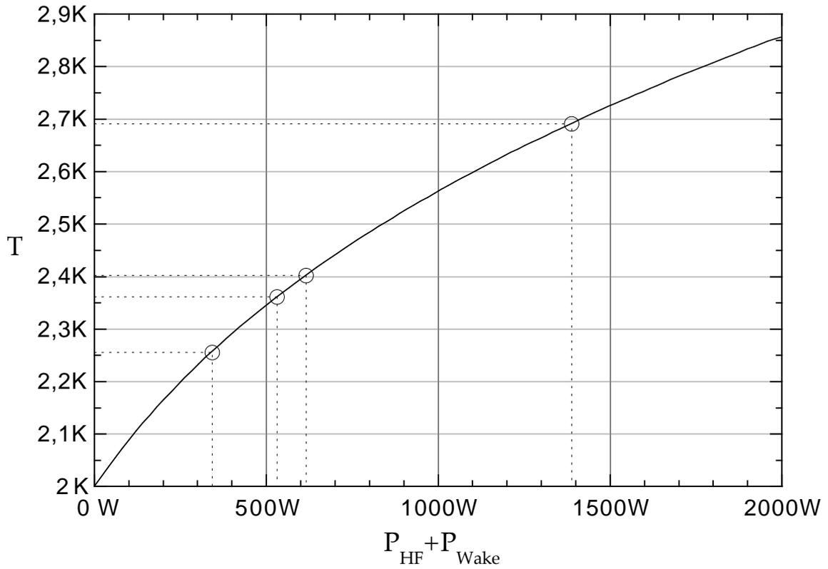
Fig. 9: Temperature at the inner surface versus the power dissipated in a nine cell cavity (RRR=300).
