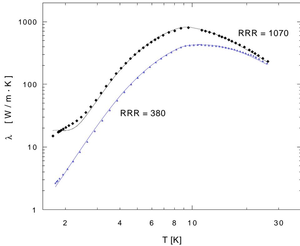
Fig. 8: Heat conductivity versus temperature for niobium.
