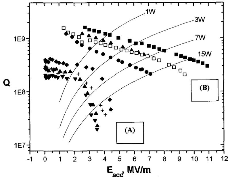
Fig. 2.4 Group (A) represents those cavities which are currently installed in ALPI and operating since 1995: these  $Q_0$  values were as low also in off-line tests, the reason being an inconvenience which occurred during sputtering. Group (B) shows the present off-line state-of-the-art: accelerating fields ranging between 5.8 and 8 MV/m can be achieved without field emission drop and with the same reliable sputtering recipe (the field limiting phenomenon is a general warm-up of the resonators).
