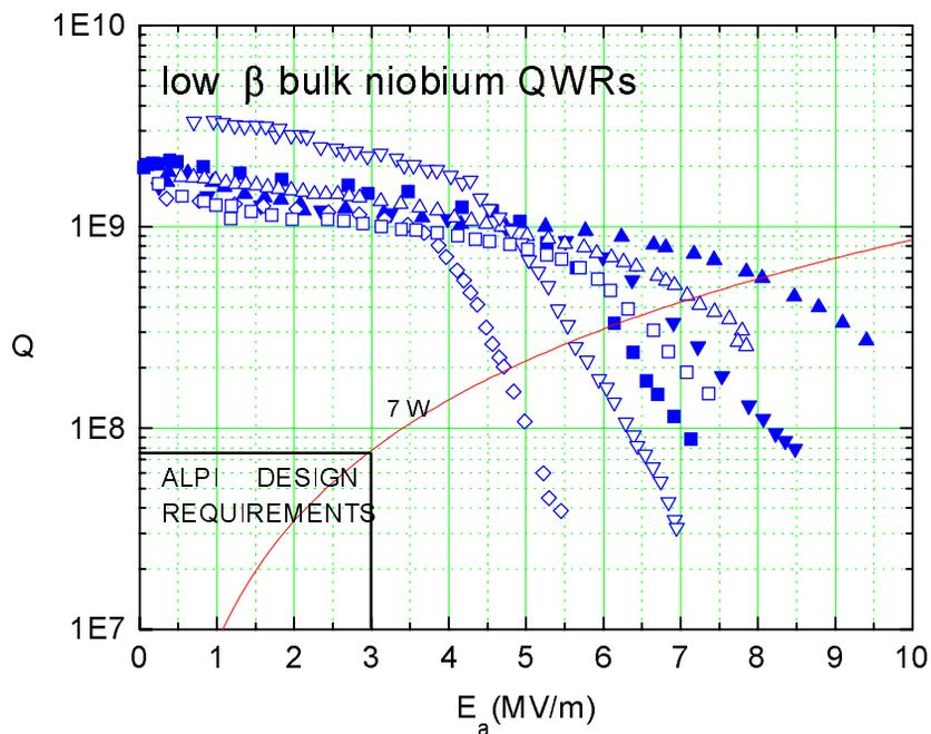
Fig. 2.2  $Q_0$  vs.  $E_a$  fields of LNL full Nb QWR's. It can be noted that the cavity reaching the higher  $Q_0$  drops at lower fields, while the resonator reaching 8 MV/m at 7 W was high pressure rinsed, a phenomenon which is known to slightly reduce  $Q_0$  at low fields but to push the FE limitation to higher fields
