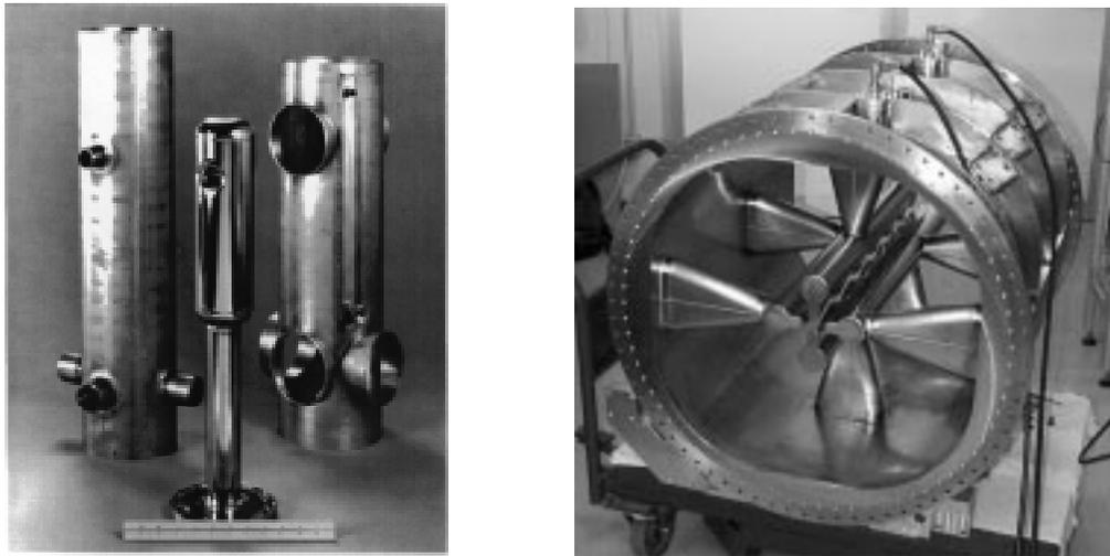
Fig. 2.3 Full Nb low- $\beta$  cavities are favoured in case of complicated geometry. The New Delhi/Argonne modified QWR and the being built LNL superconducting RFQ are shown as examples.
