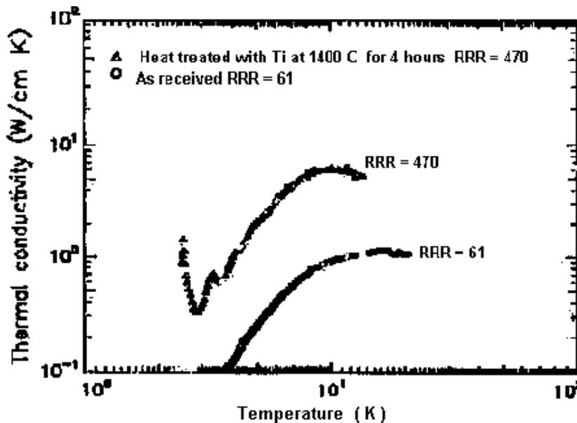
Fig 1 The thermal conductivity of Chinese Nb sheet
