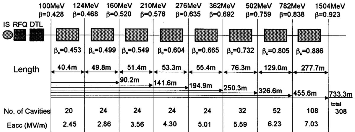
Fig.1 Preliminary conceptual design of the superconducting linac.
