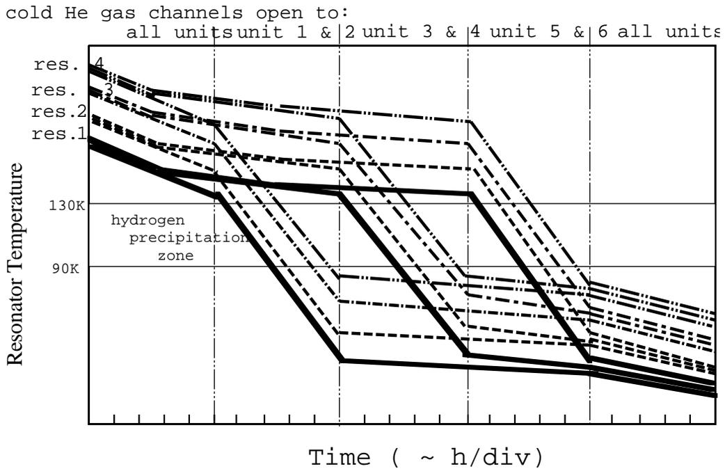
Fig. 5 Scheme of a two-units(cryomodules)-by-two-units sequential precooling over the hydride precipitation zone of 130 K to 90 K.
