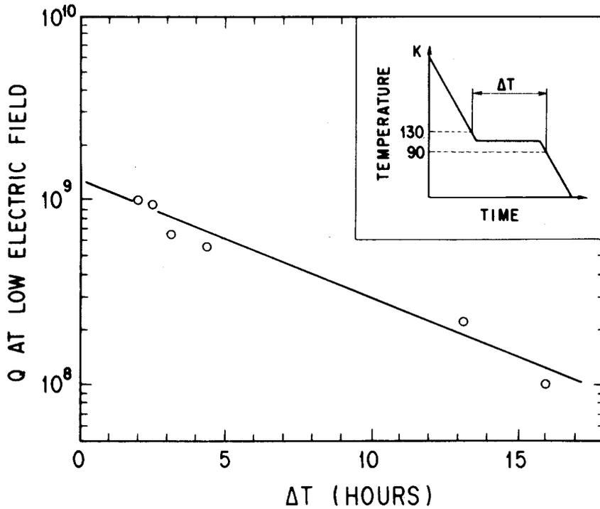
Fig.4 Q-degradation on cooling between 130 and 90K. Q-factors at low fields are plotted as a function of holding time between 130 and 90 K[6,10].
