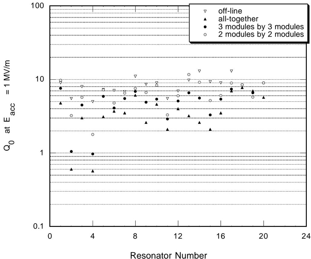
Fig.6 Q-recovery by sequential fast precooling modes
