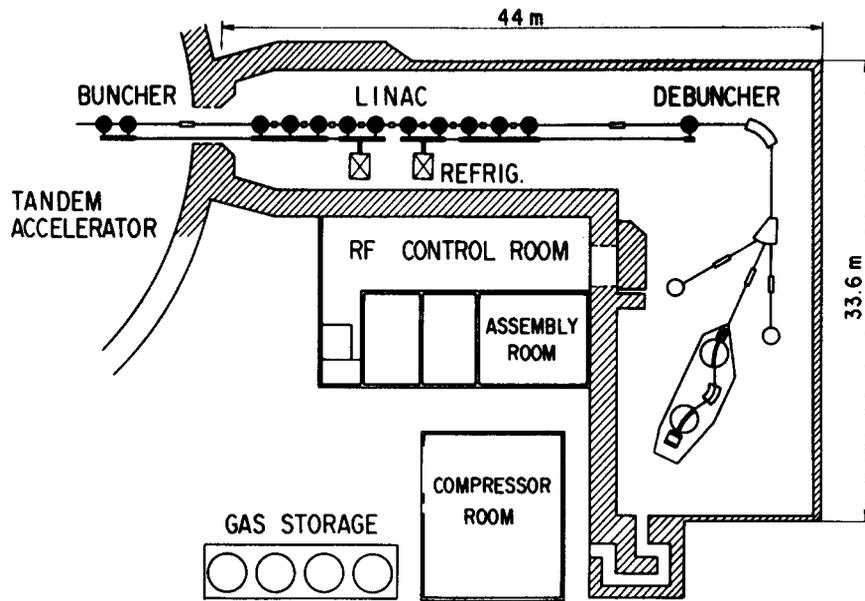
Fig.1 Layout of the JAER tandem booster
