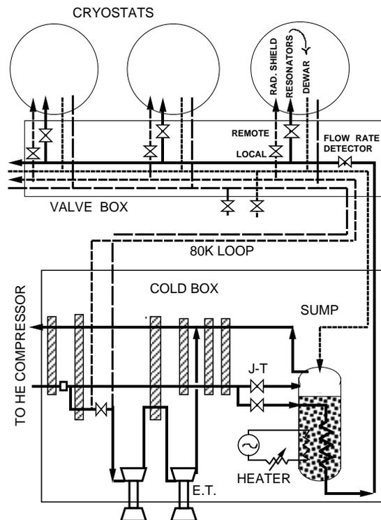
Fig.3 Flow scheme of the 4.5 K and 80 K loops in the cryogenic system
