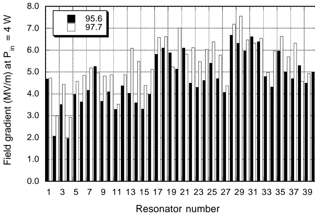
Fig. 8 Accelerating field gradients of the booster linac QWRs at the RF input of 4 W, measured in 1995 and 1997.
