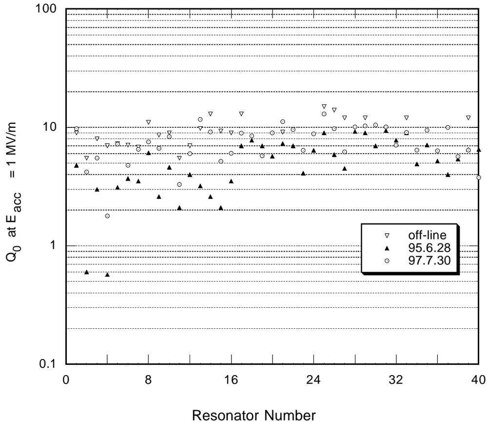
Fig.7 Q factors of the booster linac superconducting quarter wave resonators measured in 1995 and 1997 as well as in the off-line tests.
