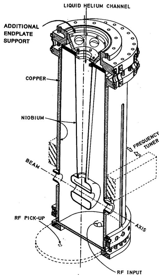
Fig. 2 129.8 MHz superconducting quarter wave resonator with  $\beta = 0.1$
