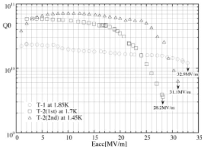
Fig.2 Q<sub>0</sub>-E<sub>acc</sub> plots on single-cell cavities No X-ray was observed up to the maximum field.
