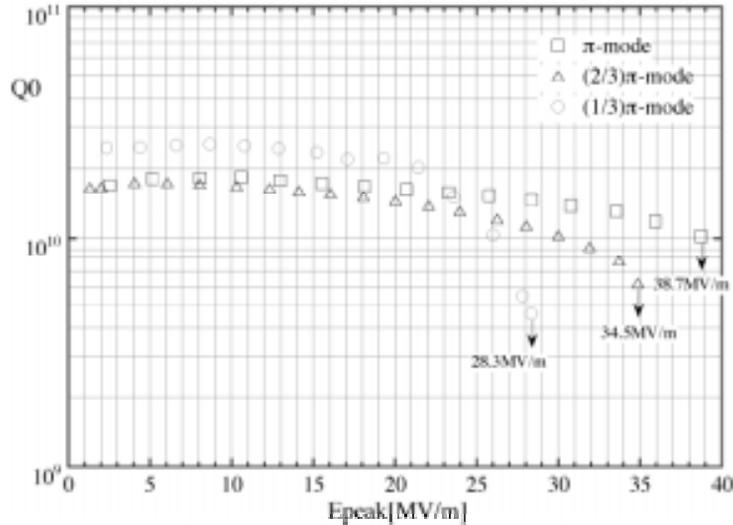
Fig.4  $Q_0$ - $E_{\text{peak}}$  plots of each mode on three-cell cavity
