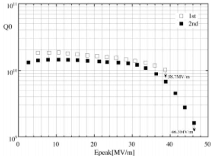
Fig.5  $Q_0$ - $E_{\text{peak}}$  plots on three-cell cavity
