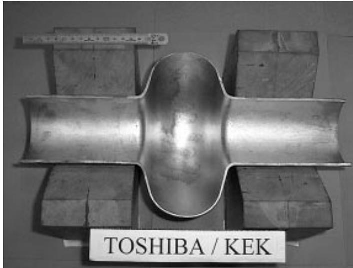
Fig.7 L-band copper cavity by hydroforming
