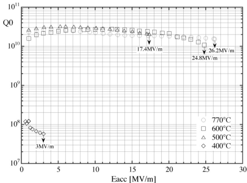
Fig.6  $Q_0$ - $E_{\text{acc}}$  plots on single-cell cavity for various annealing temperature
