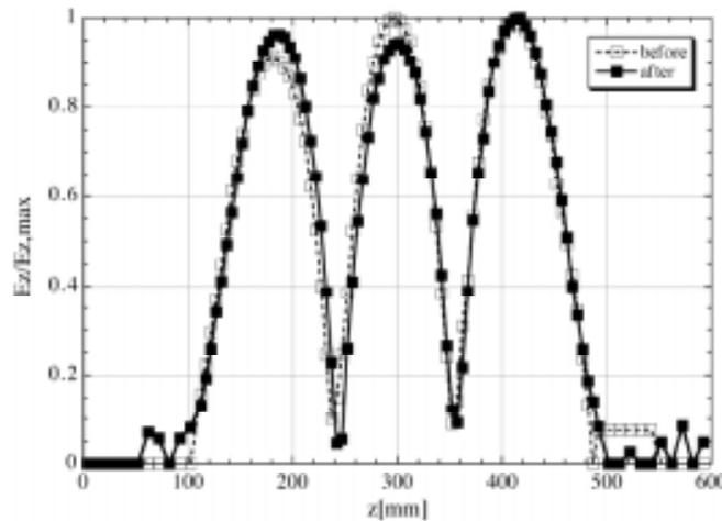
Fig.3 Electric field distribution after pre-tuning for three-cell cavity
