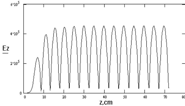
Fig. 5. The accelerating field amplitude along the cavity axis.
