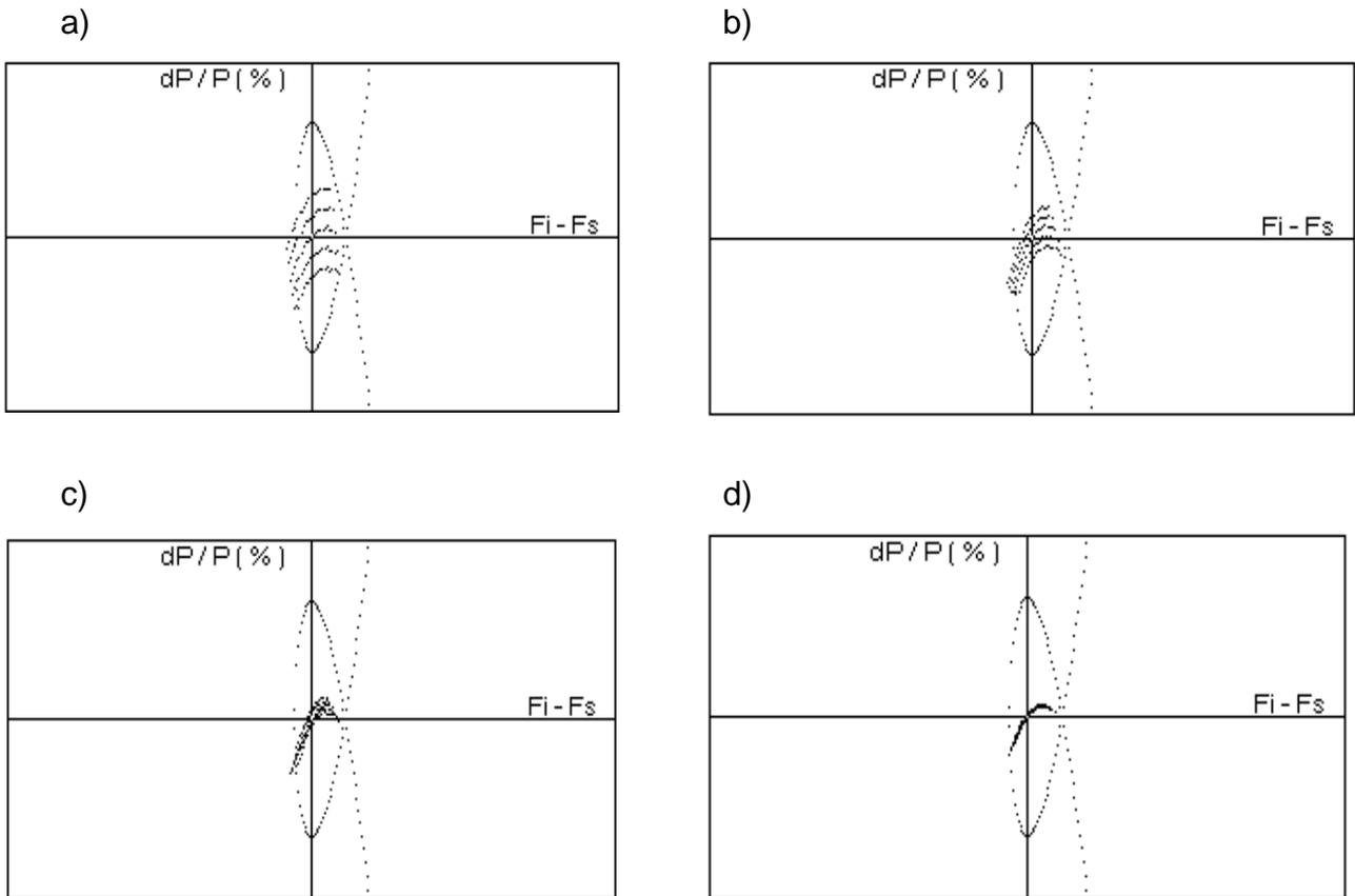
Fig. 6. The beam longitudinal phase portrait at the  $(dP/P, \varphi - \varphi_s)$  - plane on the background of separatrice for injection energy 250 keV: a) - cell No 1,  $E=0.389$  MeV,  $L=0.039$  m; b) - cell No 3,  $E=0.636$  MeV,  $L=0.082$  m; c) - cell No 5,  $E=1.373$  MeV,  $L=0.176$  m; d) - cell No 14,  $E=5.262$  MeV,  $L=0.669$  m.
