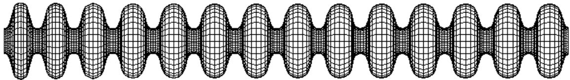
Fig. 3. The accelerating RF structure geometry of 14 cells at the injection energy 250 keV.
