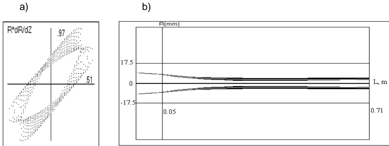
Fig. 7. The transverse dynamic simulation for SVAAP: a) - phase ellipse on the  $(R, R')$ -plane; b) - the beam trajectories along focusing channel.
