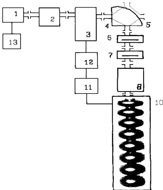
Fig. 1. The topological scheme of SVAAP: 1 - injector, 2 - electron-optical focusing system, 3 - prismatic chopper cavity, 4 - collimating slot, 5 - bending magnet, 6, 7 - collimating slots, 8 - electrostatic lens, 9 - SC accelerating cavity, 10 - cryostat, 11, 12 - RF feed system of SC cavity and chopper cavity.
