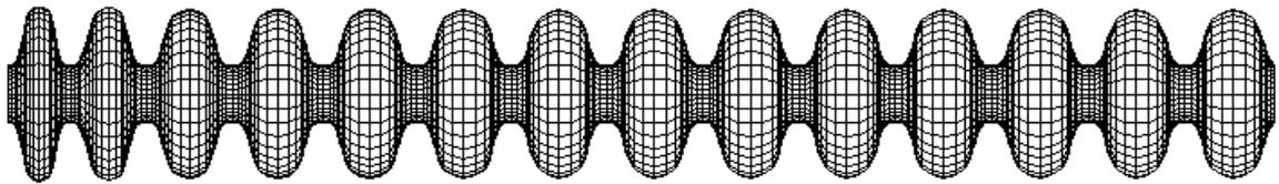
Fig. 2. The accelerating RF structure geometry of 14 cells at the injection energy 50 keV.
