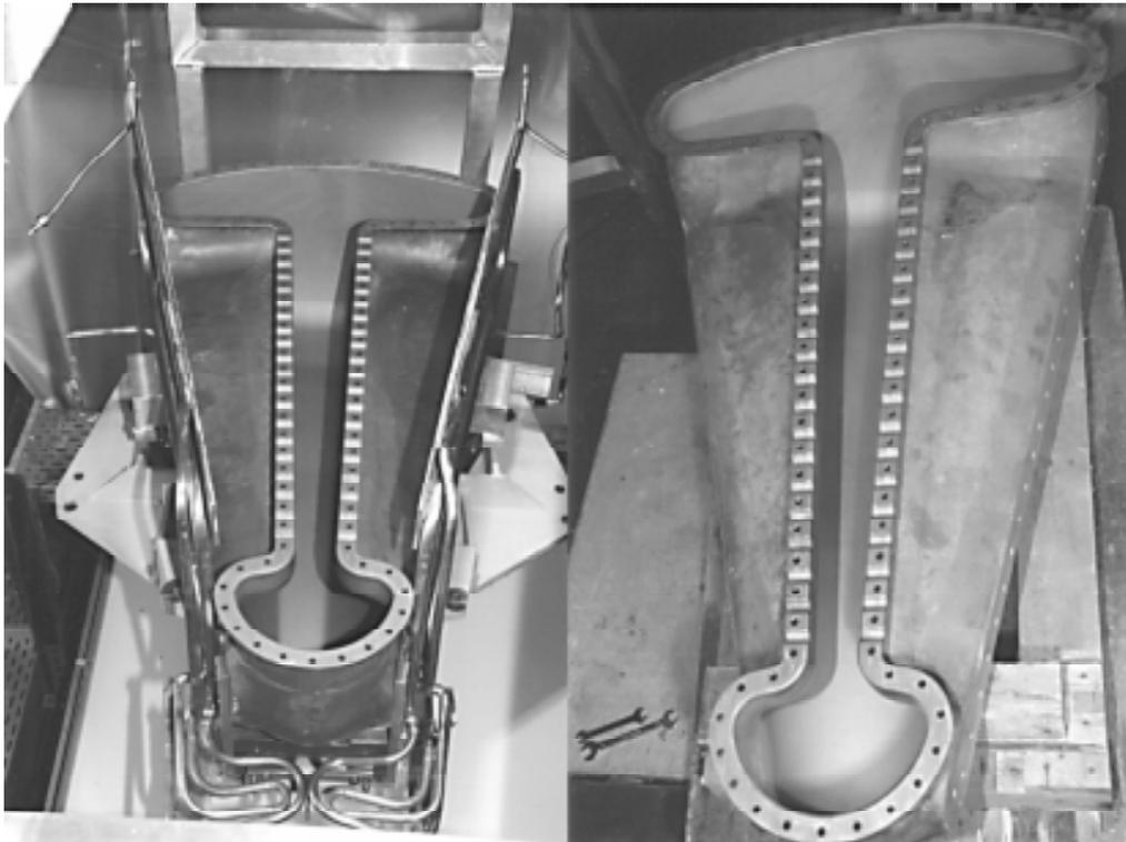
Figure 2. Two halves of a cavity, the left showing the O-shaped cooling pipes on both sides attached. The cavities (see Figure 2) are described in detail elsewhere (5). They are produced by an electroforming technique from copper and then electroplated with a thin layer ( $<5 \cdot 10^{-3}$  mm) of  $Pb_{96}Sn_4$ , which becomes superconducting below 7.5 K. Each cavity consists of two halves,
