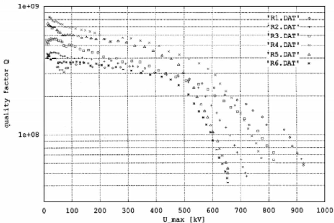
Figure 3. Quality factors of the six cavities versus the voltage amplitude at the last beam hole, with the antennas strongly coupled as under realistic beam conditions.
