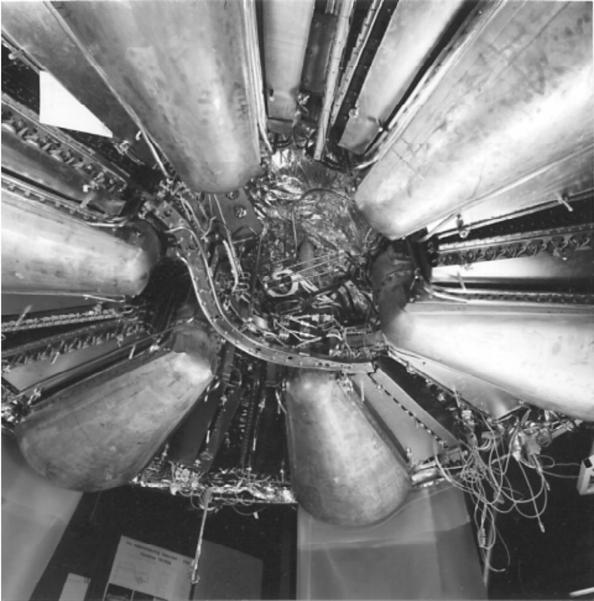
Figure 4. View from below into the TRITRON cryostat with the complete machine assembled.
