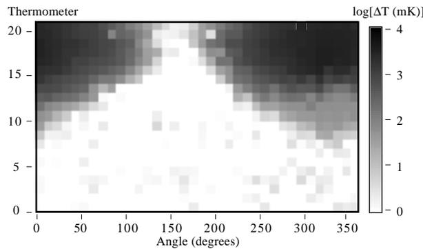
Figure 8: Cavity quench due to inadequate cooling by the helium bath of cavity LE1-33. The bath level at this time was roughly at the height of the equator (thermometer 10). Note the logarithmic temperature scale.
