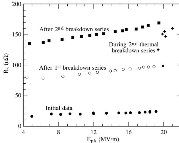
Figure 3: Surface resistance at the circled site in Figure 2 during and following a series of thermal breakdown events in the cavity.
