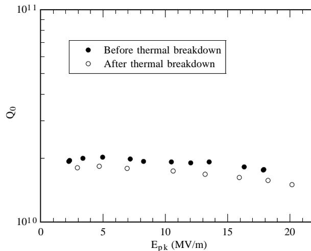
Figure 4:  $Q_0$  versus  $E_{pk}$  data obtained from power measurements on cavity LE1-32, prior to and after thermal breakdown events like those in Figure 1.
