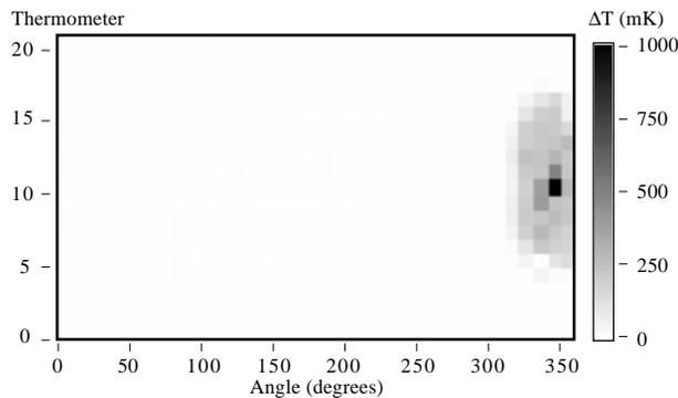
Figure 1: “Flattened” temperature map of defect initiated thermal breakdown in progress in cavity LE1-32. The bottom and top cavity irises are at thermometer 1 and 19, respectively, and the equator is at thermometer 10.
