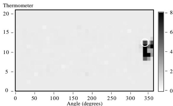
Figure 2: Ratio of the surface resistance (at  $E_{pk} = 10$  MV/m) after several breakdown events in cavity LE1-32 to that before breakdown. Dark regions indicate that the surface resistance increased.
