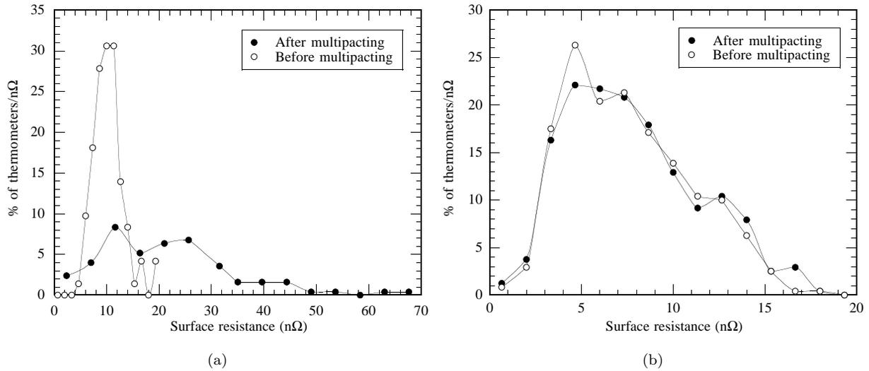
Figure 7: Histogram of  $R_s$  of sites in cavity LE1-21 covered by (a) the equator thermometers and their nearest neighbors, and (b) the thermometers away from the equator. In (a) the mean surface resistance increased from 10.3 nΩ to 21.4 nΩ following a series of breakdown events whereas in (b) the mean surface resistance did not change significantly.
