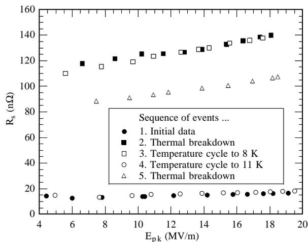
Figure 5: Surface resistance recorded by thermometer 11 at  $330^\circ$  with cavity LE1-32 (just below the circled site in Figure 2). The data was obtained in the following sequence: 1. before any thermal breakdown, 2. following a series thermal breakdown events, 3. following a thermal cycle to 8 K, 4. following a second thermal cycle to 11 K, and 5. following a new series of thermal breakdown events.
