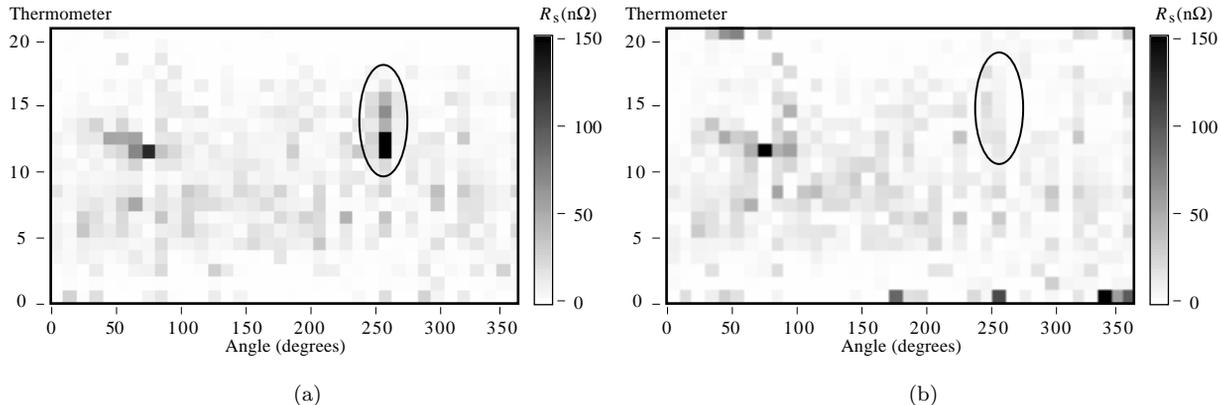
Figure 9: Map of the surface resistance of cavity LE1-33 at  $E_{pk} = 12$  MV/m. (a) Before the quench in Figure 8 occurred, and (b) after the quench. The circled region had previously increased its surface resistance due to defect related thermal breakdown.
