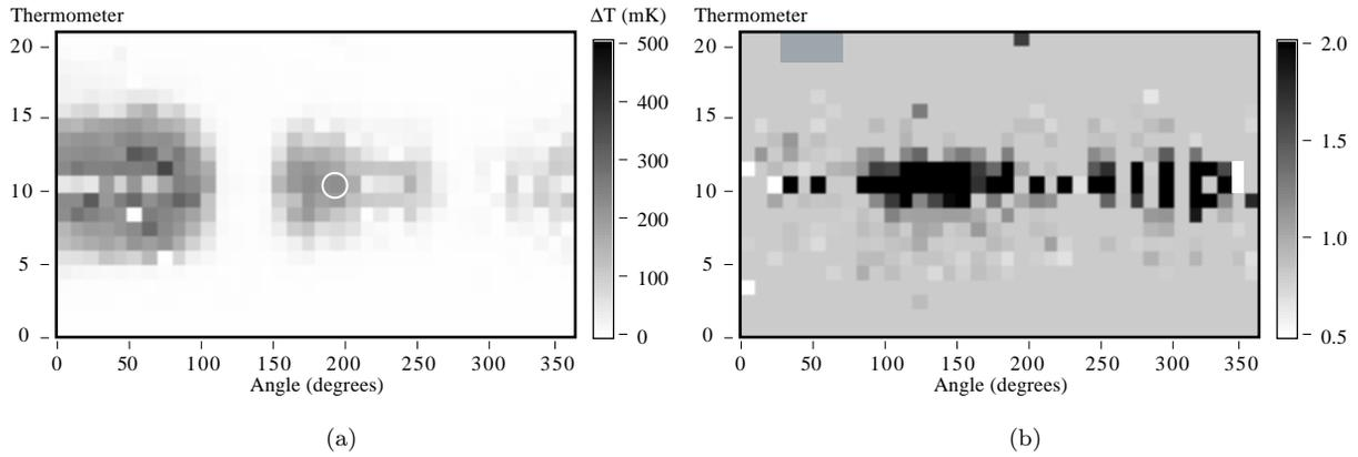
Figure 6: (a) Temperature map taken during a test of cavity LE1-21 while multipacting was active at  $E_{pk} \approx 34$  MV/m. (b) Ratio of the cavity's surface resistance after and prior to multipacting, depicting increased losses along the equator.
