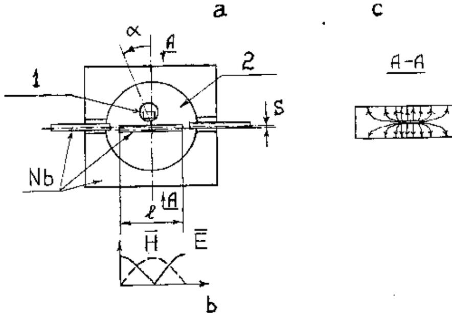
**Figure 1.** Scheme of the measuring microstrip niobium resonator. (a) Top view: 1 - sample, 2 - teflon disk; (b) Spatial distribution of electromagnetic field amplitudes along the resonator; (c) Configuration of the field line in the cross-section.
