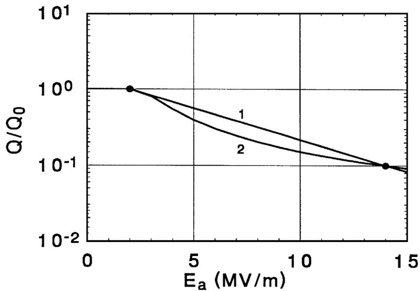
Figure 2: Dependence of the normalized Q-value  $Q/Q_0$  on the field amplitude  $E_a$ , in the field of non-quadratic losses. The dependence approximate to the experimental data is marked 1. The calculated dependence (15) is normalized on the experimental data • and marked 2.
