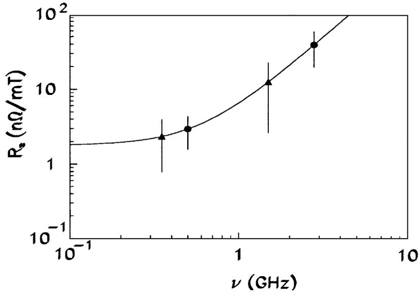
Figure 1: Dependence of the NbCu cavities resistance (14) normalized on the field amplitude  $B_a$  on frequency  $\nu$ . The dependence is normalized on the data at  $\nu = 0.5 \text{ GHz}$  and  $\nu = 2.79 \text{ GHz}$ —•.
