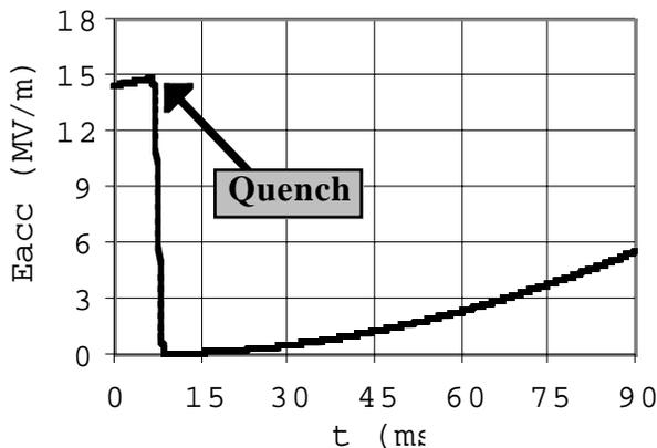
**Fig. 7:** Variation of  $E_{acc}$  during a quench in a 3 GHz cavity.
