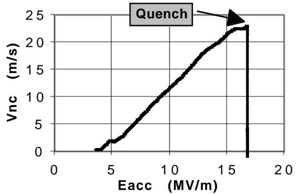
**Fig. 14:** Expansion velocity as a function of the accelerating field.
