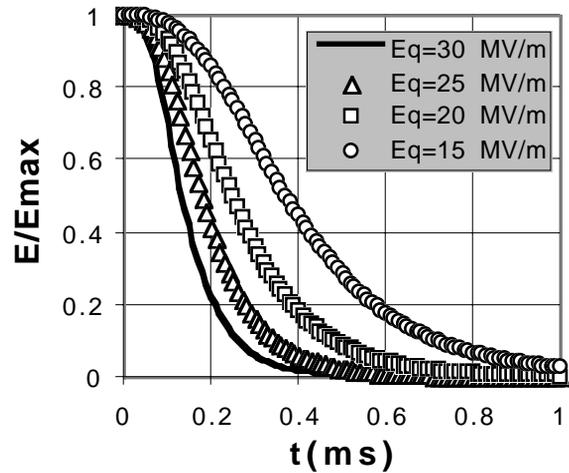
**Fig. 17:**  $E_{acc}$  decrease during a quench for different quench fields.
