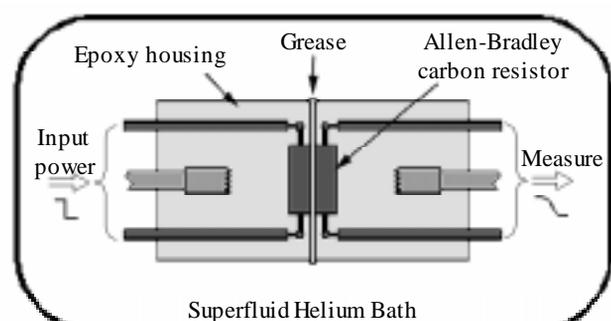
**Fig. 2:** Scheme of the experiment with the Cornell thermometers.
