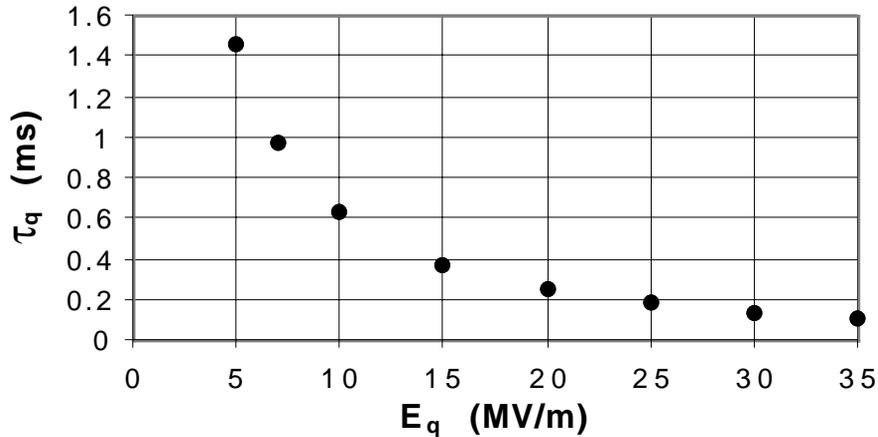
**Fig. 18:** Time constant  $\tau_q$  as a function of the quench field.
