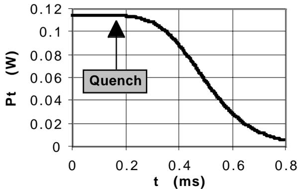
Fig. 9: Typical transmitted power recorded during a 3 Ghz cavity quench.
