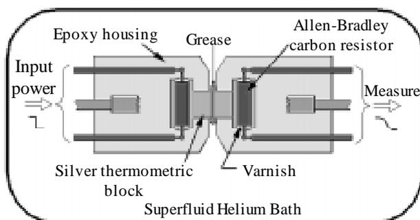
**Fig. 1:** Scheme of the experiment with the IPN thermometers.
