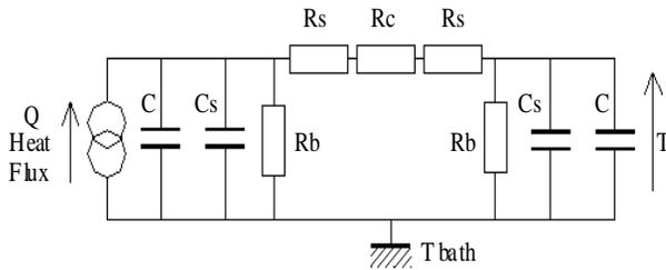
**Fig. 5:** Equivalent electrical scheme for the IPN thermometers.
