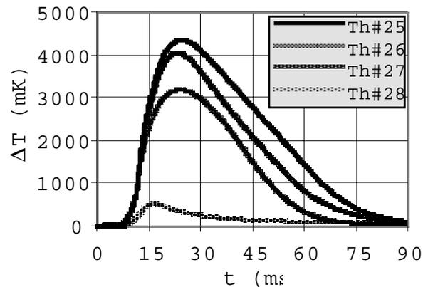
**Fig. 8:** Heatings measured on 4 thermometers during the quench.
