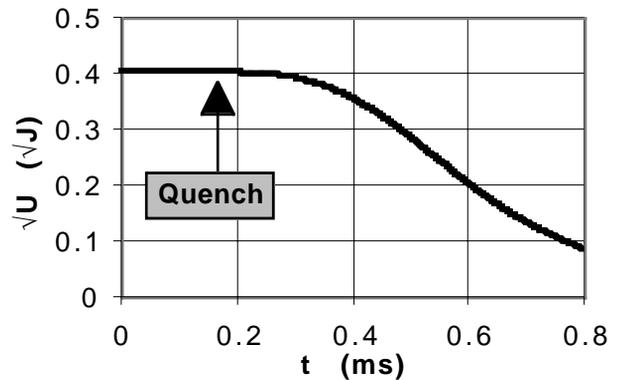
Fig. 10: Square root of the stored energy during the quench.
