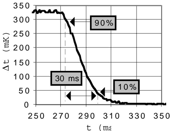
**Fig. 3:** IPN thermometer response to a pulsed power at  $T=1.8$  K.
