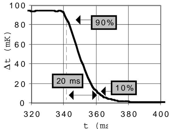
**Fig.4:** Cornell thermometer response to a pulsed power at  $T=1.8$  K
