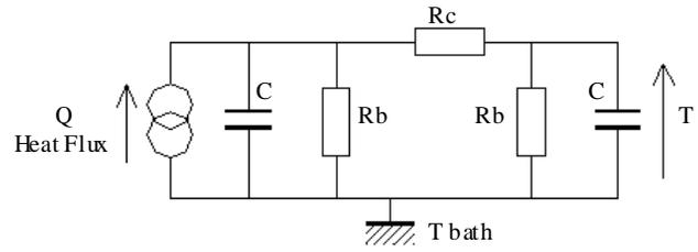
**Fig. 6:** Equivalent electrical scheme for the Cornell thermometers.
