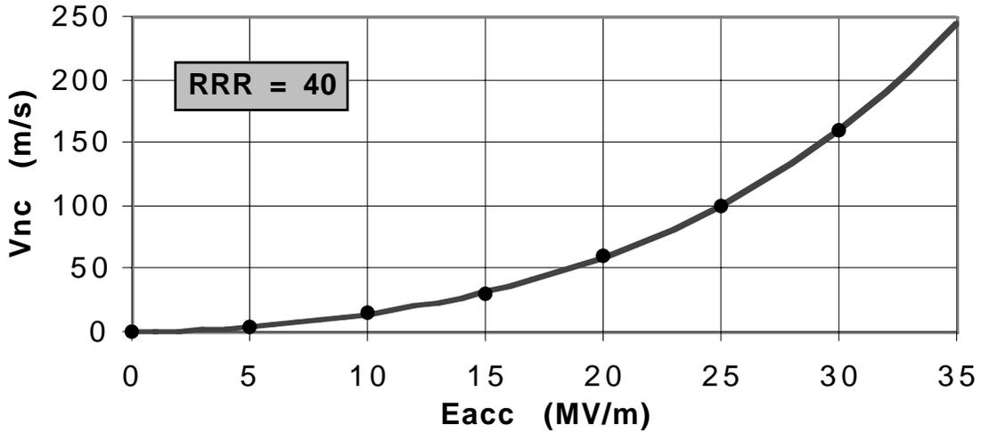
**Fig. 15:** Calculated expansion velocity as a function of  $E_{acc}$ .
