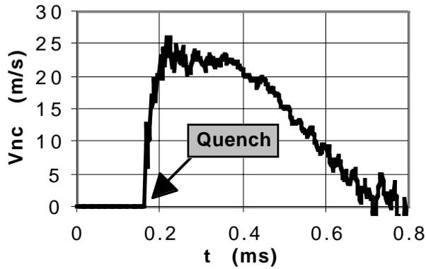
**Fig. 13:** Expansion velocity of the normal conducting area.
