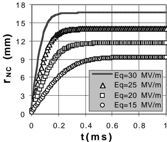
**Fig. 16:** Calculated normal region radius for several quench fields.
