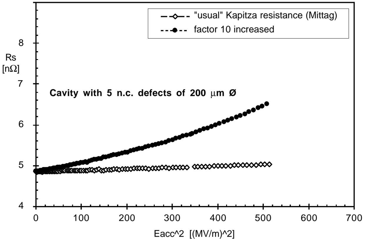
Fig.10: Calculated increase of the surface resistance versus the squared accelerating field (RRR=525, T=1,8K)
