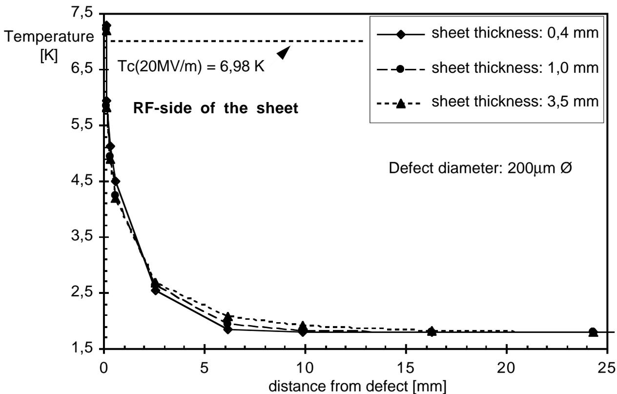
Fig.7: Radial temperature profile at  $E_{acc}=20\text{MV/m}$  for different sheet thickness ( $T=1,8\text{K}$ ,  $\text{RRR}=525$ )
