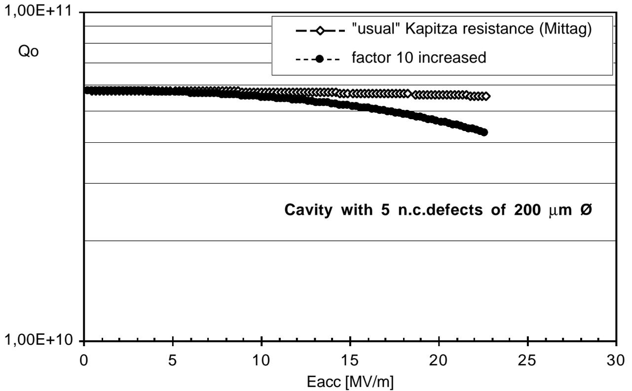
Fig.9: Comparison of  $Q_0(E_{acc})$ -dependance for a factor 10 increased Kapitza resistance (RRR=525, T=1,8K)
