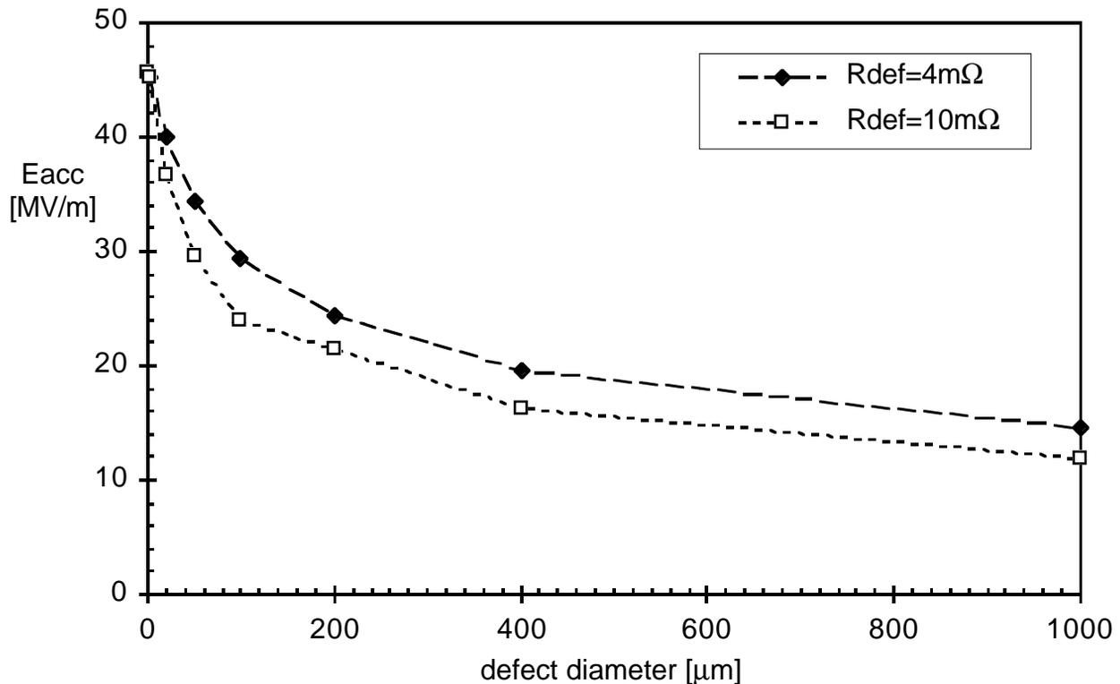
Fig.3: Calculated breakdown limit for different surface resistances  $R_{\text{def}}$  of the defect ( $\text{RRR}=525$  ;  $T=1,8\text{K}$ )
