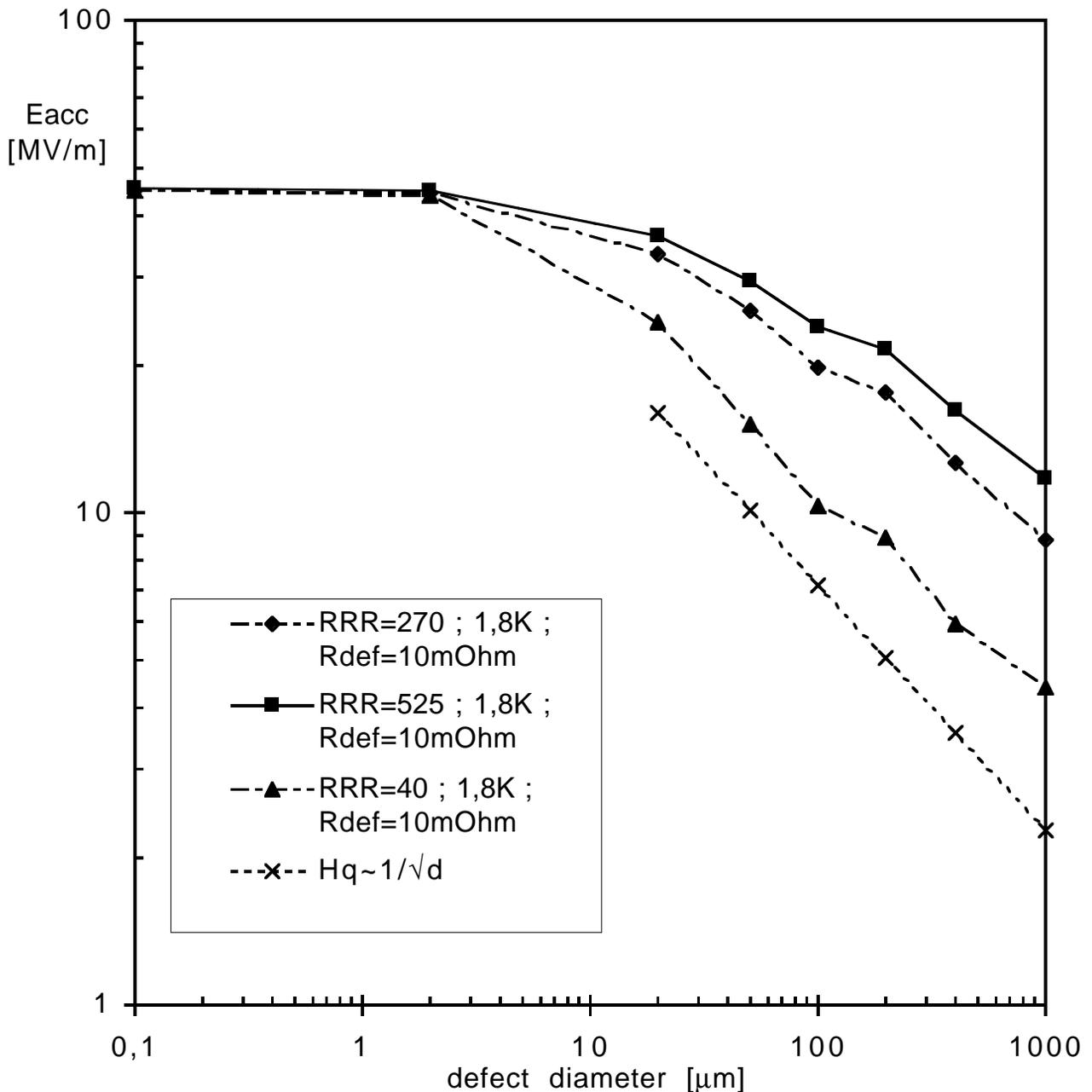
Fig.2: Calculated breakdown field for RRR=525, RRR=270 and RRR=40. The analytical  $Hq \sim 1/\sqrt{d}$  is shown as comparison.
