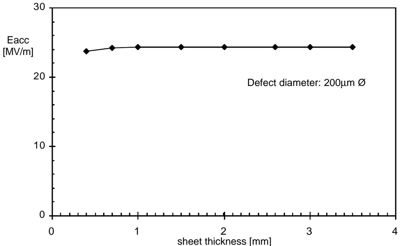
Fig.5: Quench limit as a function of the sheet thickness for a defect diameter of 200 $\mu$ m (RRR=525, T=1,8K)
