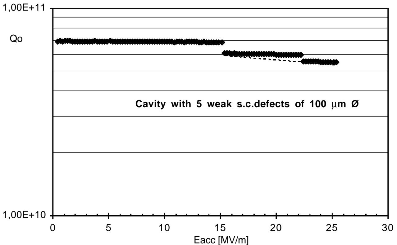
Fig.13: Calculated  $Q_0(E_{acc})$  of a cavity with 5 weak superconducting defects of  $100 \mu\text{m } \emptyset$  (RRR=525 ;  $T=1,8 \text{ K}$  ;  $R_{def}(T > T_c)=10 \text{ m}\Omega$ )
