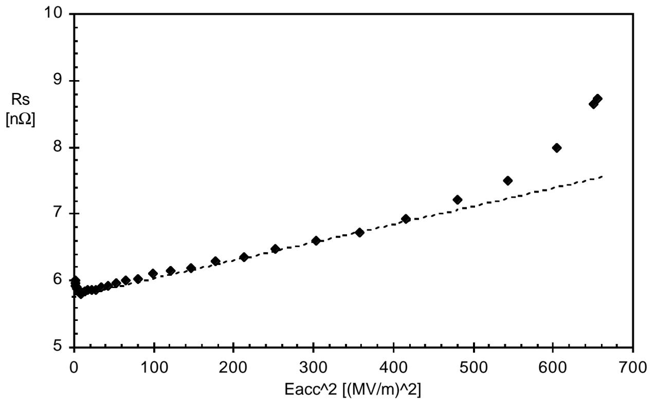
Fig.12: Quadratic increase of the surface resistance at the same test
