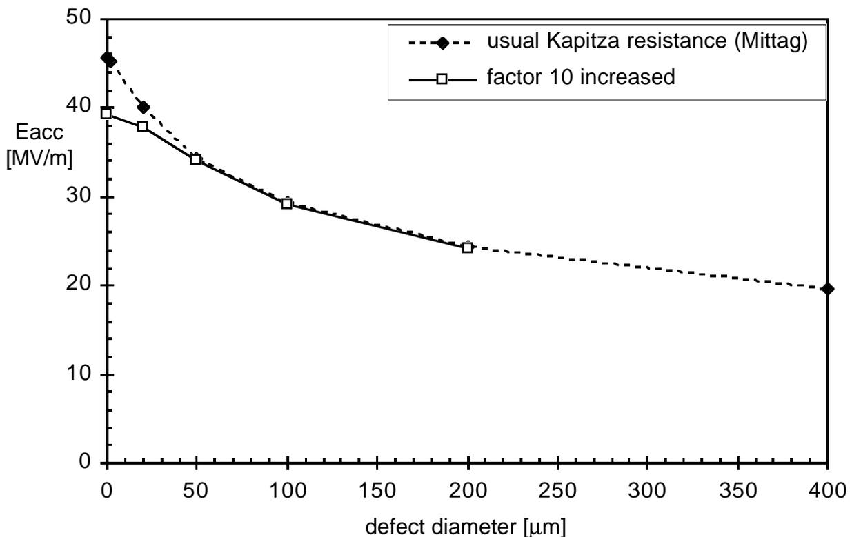
Fig.8: Comparison of breakdown limits for a factor 10 increased Kapitza resistance (RRR=525,  $T=1,8\text{K}$ ,  $R_{def}=4\text{m}\Omega$ )
