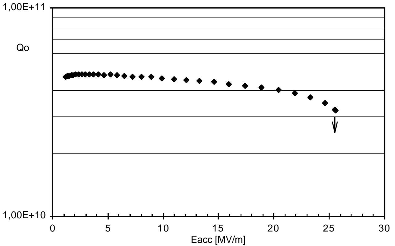
Fig.11: Measured  $Q_0(E_{acc})$ -performance of cavity D3 (limited by quench ;  $RRR \approx 525$  ;  $T = 1,8K$ )
