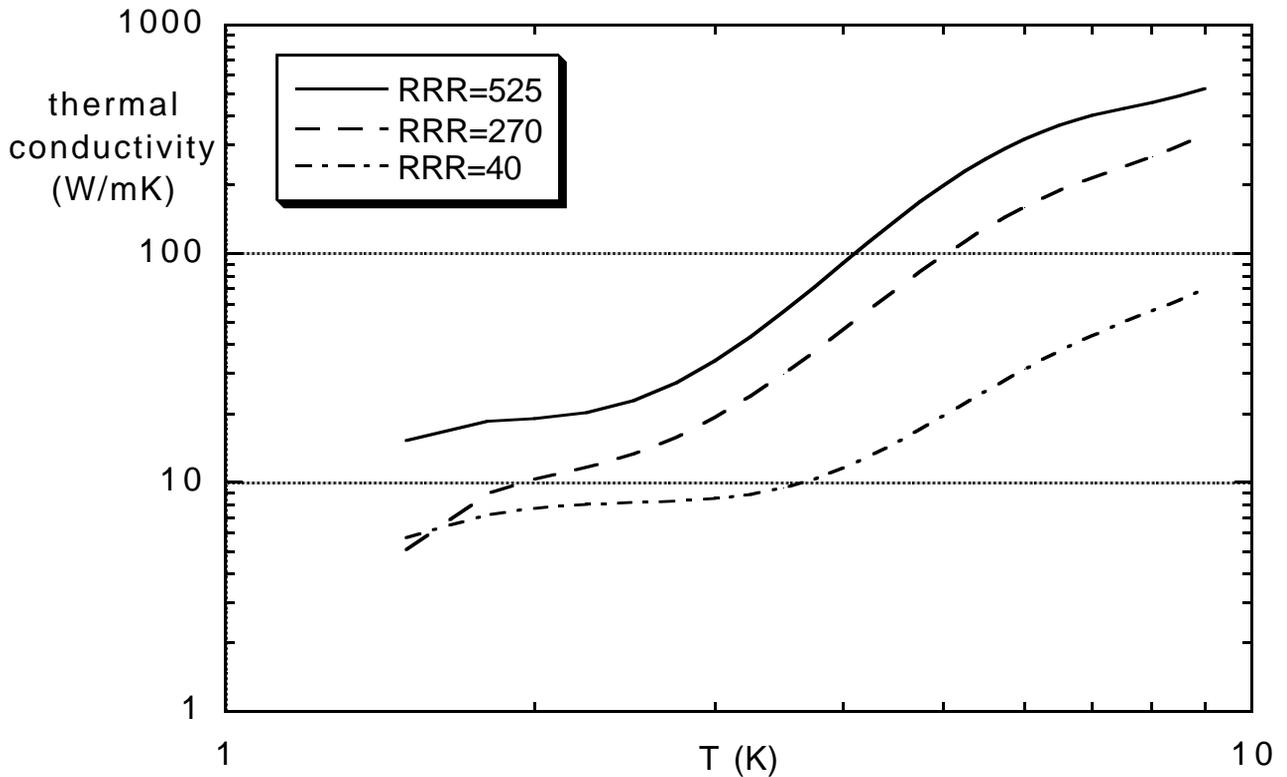
Fig.1: Thermal conductivity fits used for the calculations
