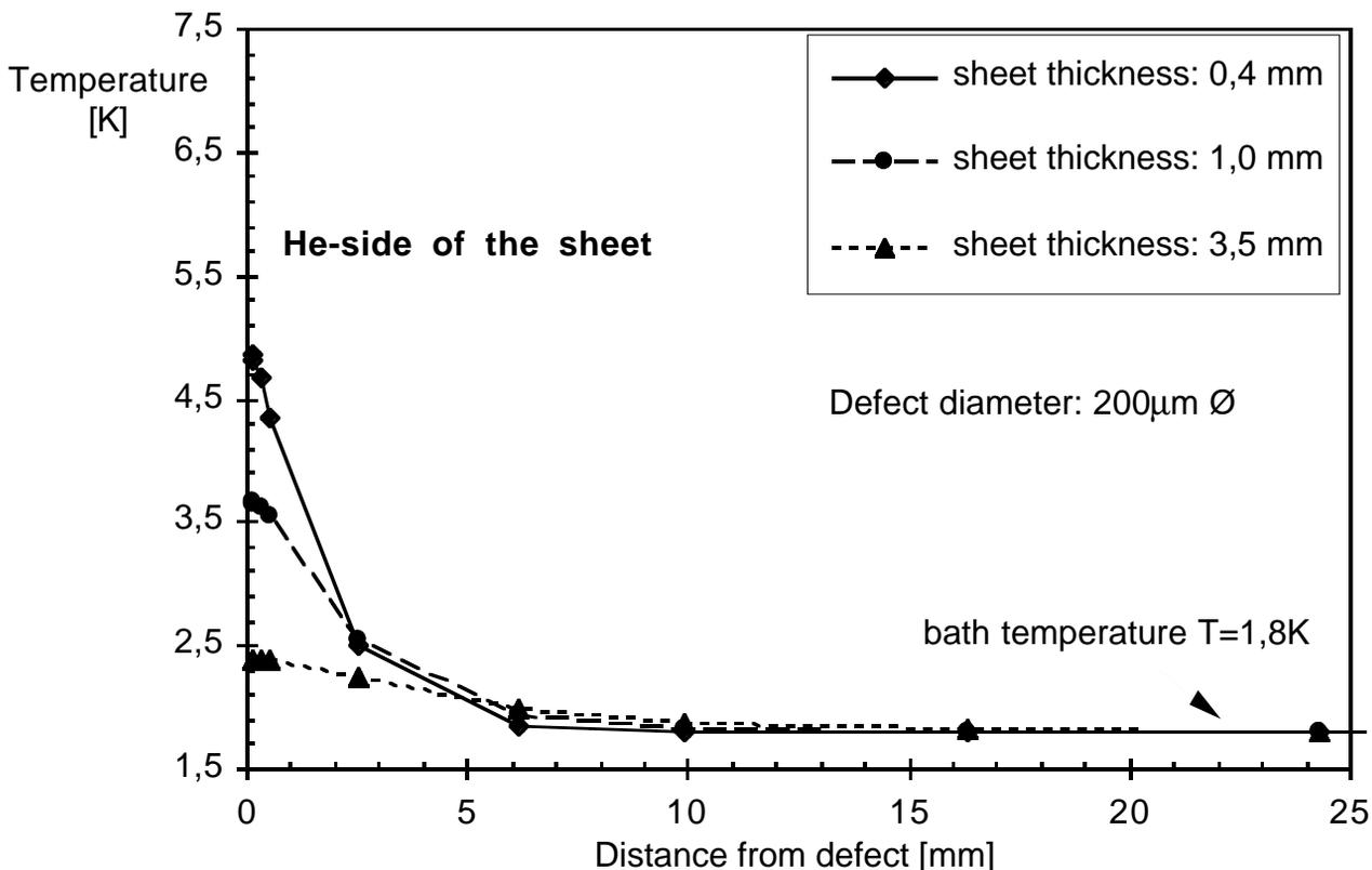
Fig.6: Radial temperature profile at  $E_{acc}=20\text{MV/m}$  for different sheet thickness ( $T=1,8\text{K}$ ,  $\text{RRR}=525$ )
