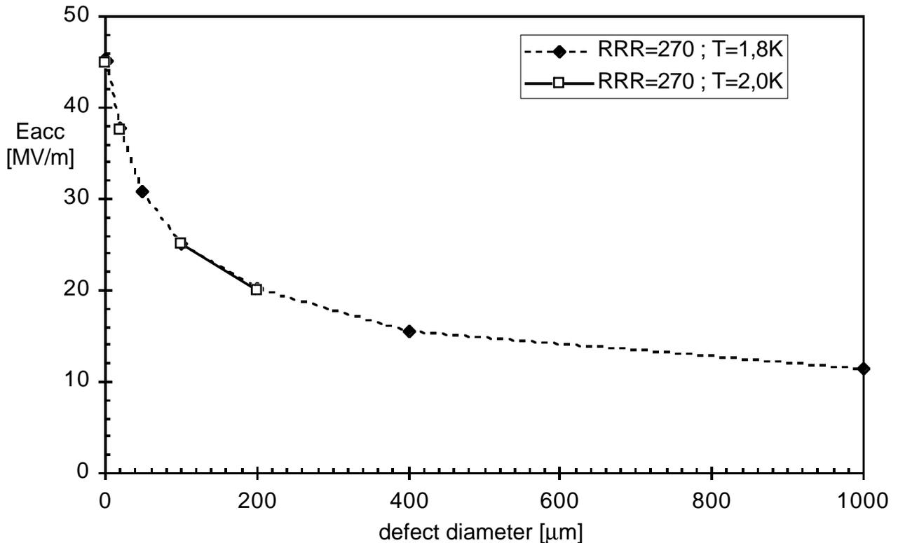
Fig.4: Comparison of breakdown limits for He bath temperature of  $T=1,8\text{K}$  and  $T=2,0\text{K}$  ( $\text{RRR}=270$ ,  $R_{\text{def}}=4\text{m}\Omega$ )
