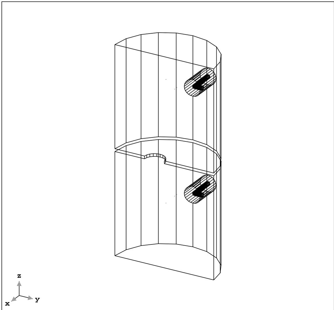
**Fig. 2. Schematic view of two coupled cylindrical cavities.**
