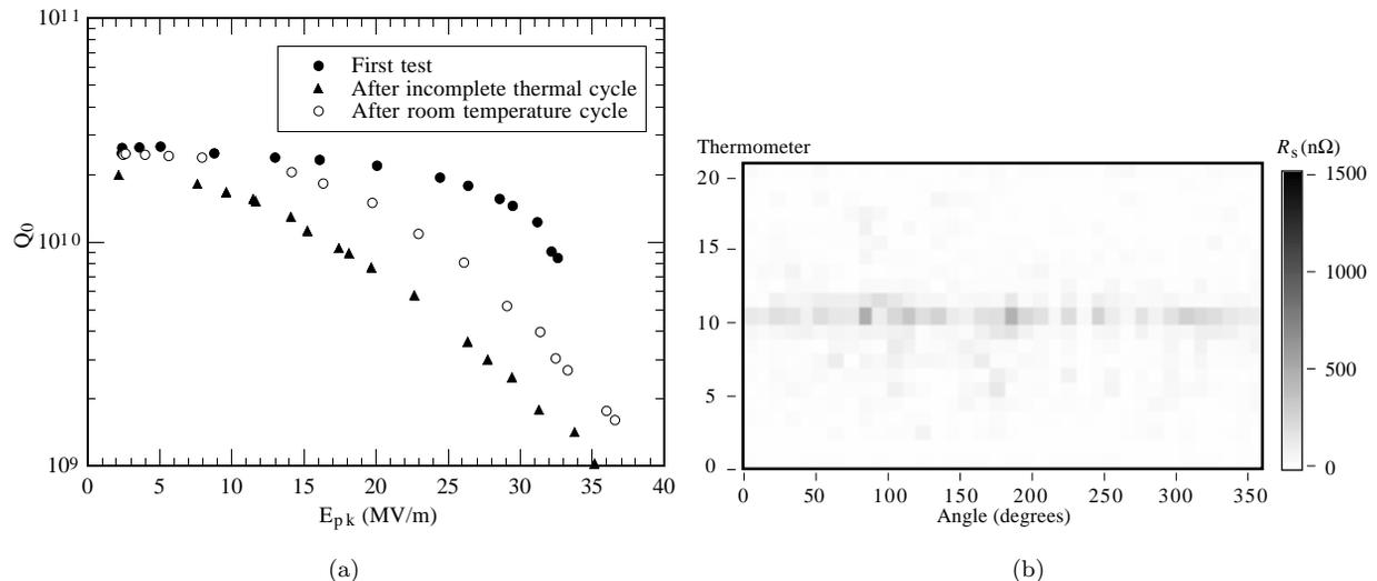
Figure 5: (a)  $Q_0$  results obtained with cavity LE1-34. In all cases, x rays were only detected at  $E_{pk} = 20\text{ MV/m}$  or higher. (b) Surface resistance of cavity LE1-34 at 30 MV/m, following an incomplete thermal cycle and then a complete cycle to room temperature.
