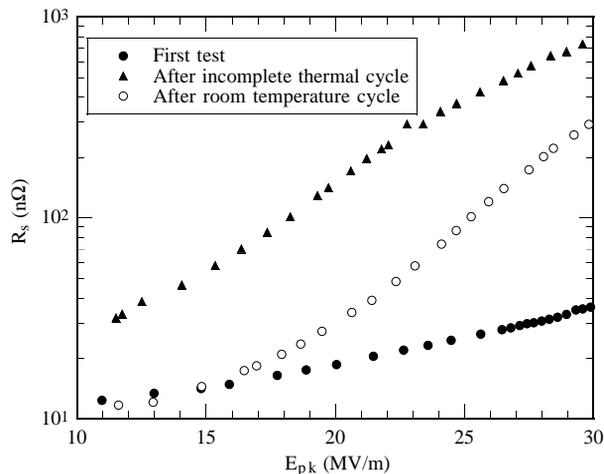
Figure 6: Surface resistance recorded at the circled site in Figure 4(a) during three different tests. The slight increase in  $R_s$  with  $E_{pk}$  during the first test was observed throughout the entire cavity and is probably not related to hydrogen contamination.
