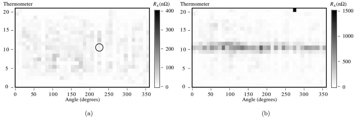
Figure 4: Surface resistance of cavity LE1-34 at 30 MV/m. (a) First test, (b) second test following a temperature cycle to  $77\text{ K} < T < 273\text{ K}$ . The losses recorded at the circled site are summarized in Figure 6.
