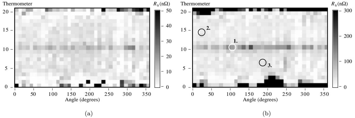
Figure 1: Surface resistance of cavity LE1-20 at (a)  $E_{pk} = 15$  MV/m and (b) 30 MV/m. The losses along the equator (thermometer 10) increase faster with  $E_{pk}$  than elsewhere, typical of hydrogen related losses. Dark regions along the irises (thermometers 1 and 19) are either field emission related, or due to noisy signals because the magnetic field is too low for reliable  $R_s$  extraction from the temperature data.
