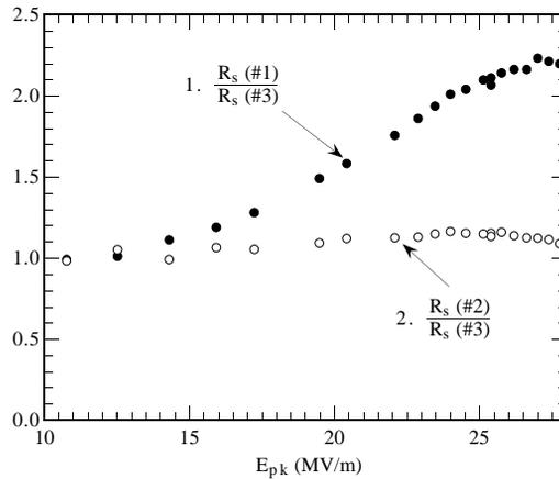
Figure 2: Ratio of the surface resistance measured by (a) thermometer “1” in Figure 1 to that measured by thermometer “3”, and (b) thermometer “2” to that measured by thermometer “3”. Both curves are normalized to one at low field.
