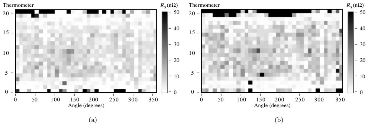
Figure 3: Surface resistance of cavity LE1-21 following a 900 °C heat treatment to remove all hydrogen. (a) At  $E_{pk} = 10$  MV/m, and (b) at 27 MV/m. No enhanced losses were observed along the equator. Dark regions along the irises are either field emission related, or due to noisy signals because the magnetic field is too low for reliable  $R_s$  extraction.
