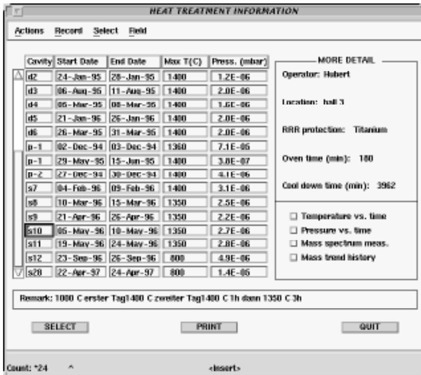
Fig. 7a: Full information from heat-treatments done on cavities
