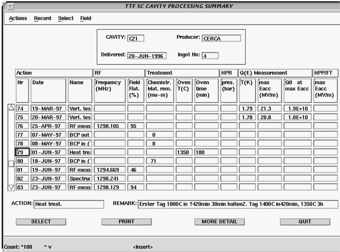
Fig. 3: Summary information from treatments and tests done on a cavity in chronological order
