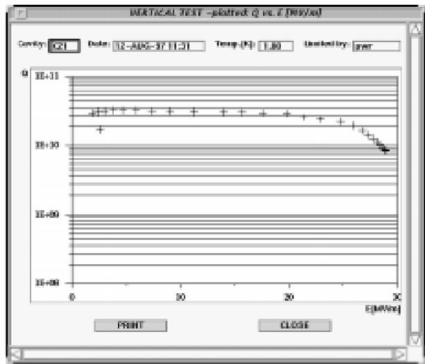
Fig. 4b: Detailed Q(E)-graph from vertical test.
