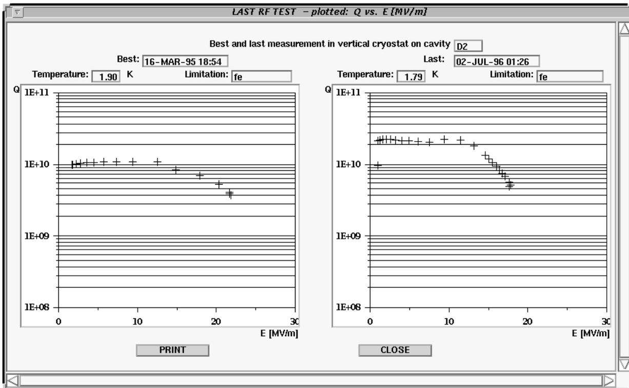
Fig. 6: Q(E)-curves of the best and last result obtained on cavity D2 in vertical tests.
